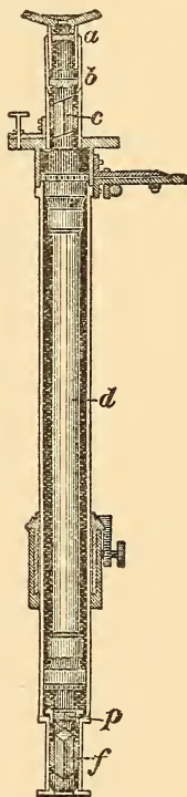
FIG. 11.—SECTIONAL VIEW OF ULZMANN'S POLARIZING SACCHARIMETER.
