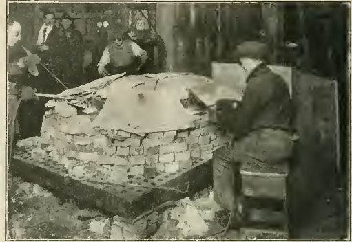
Fig. 3—Use of Preheating Furnace During Welding of Cast-Iron Piston
