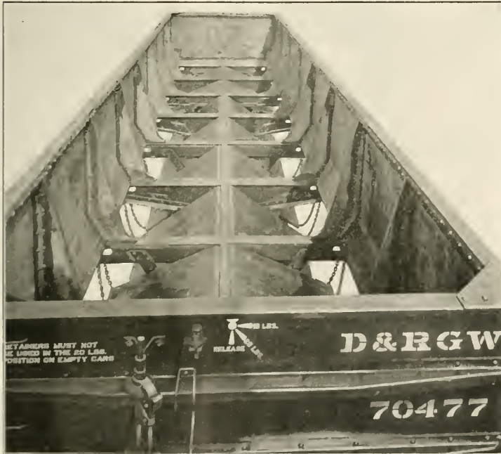
Interior of Car Showing Gussets, Doors in Open Position
