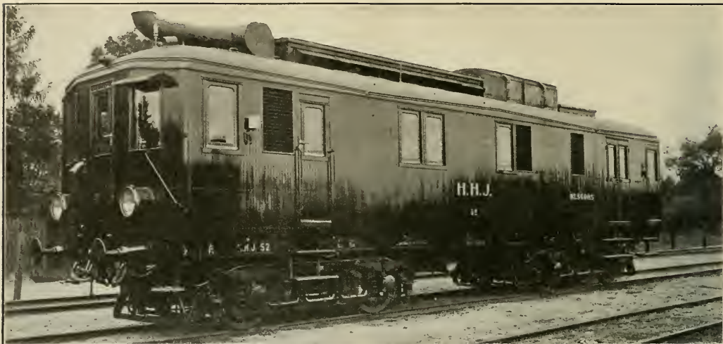
Swedish Diesel-Electric Motor Car of 250 Horsepower
