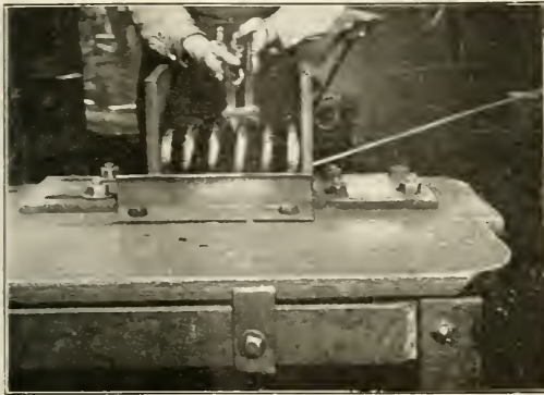
Fig. 2—Adjustable Gauge Used in Opening Springs to Standard Length
