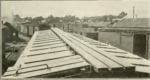
Car With Roof of Reclaimed Sheets
