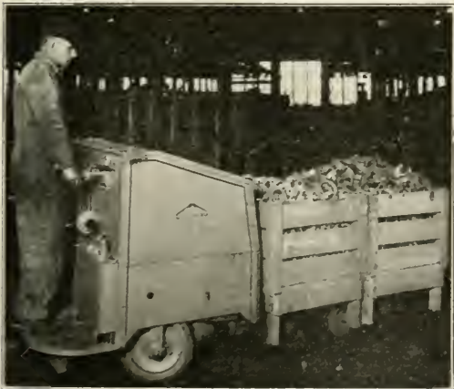
Clark Truklift with Power Elevating Platform and Compact Gasoline Motor Drive
