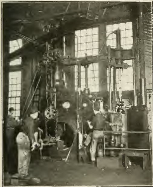
Fig. 1—300-Ton Forging Press at the Greenville Shops of the Bessemer & Lake Erie
