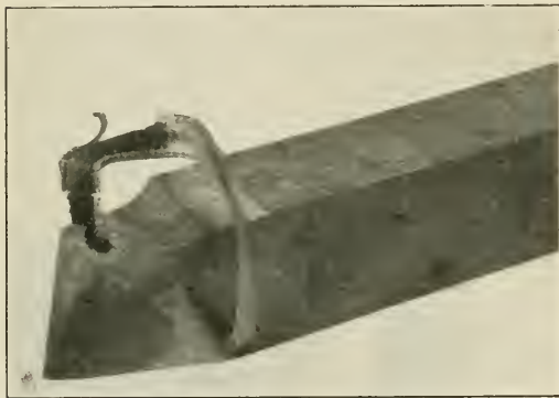
Fig. 4—"Freezing" of the Last Thin Chip to the Nose of the Tool
