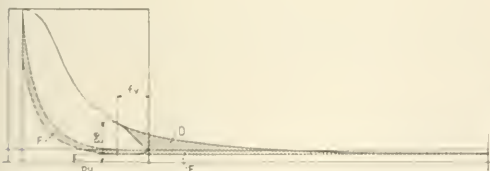
Fig. 1.—Effect of Exhaust Ejector Action on Indicator Card
