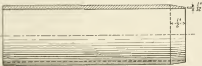
Fig. 10—Correct Method of Preparing Safe Ends for Use
