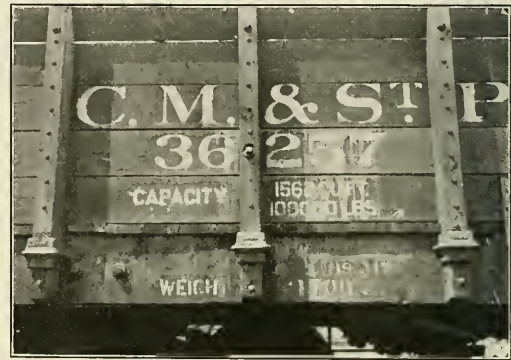
Condition of Stenciling Applied to Creosoted Surface After Eighteen Months' Service; Surface Prepared by Applying One Coat of Pure Shellac
