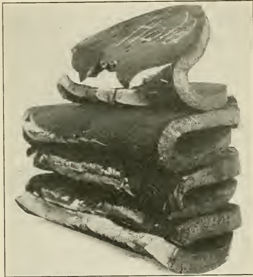
Fig. 1—Test Discs Broken with Great Difficulty After a Single Quench and Draw
