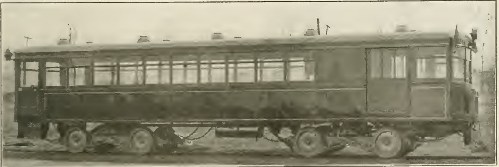
The Model 55 Service Coach Drives on All Four Wheels of the Leading Truck
