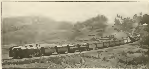
Fig. 2—Train of 360 Tons on a Heavy Grade with Two 0-8-2 Type Locomotives
