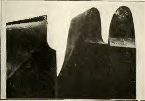
Fig. 2—Roughing Lathe Tools which Failed in Breakdown Tests
