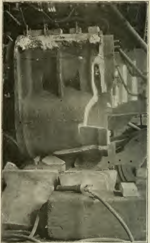
Fig. 1—Broken Locomotive Cylinder
