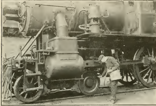
Fig. 6—Oiling a Solid Engine Truck Wheel Hub Through a Hole in the Plate
