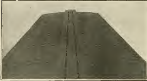
Sharon Pressed Steel Roof as Applied to the Car
