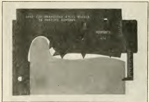
Pratt & Whitney Gage Applied to Worn Tire
