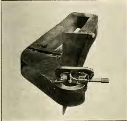
Fig. 6—Gage for Checking Roundness, and Measuring Size of Holes
