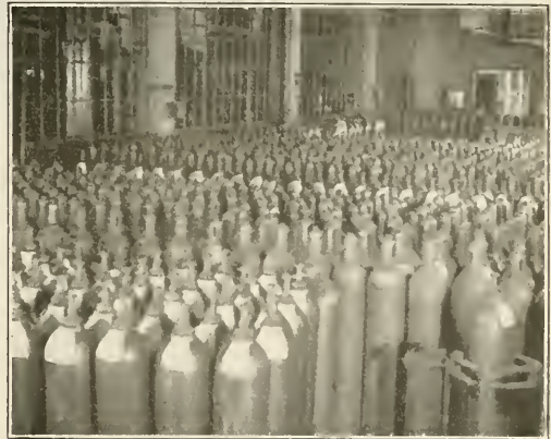
Fig. 6—Liquid Air Oxygen Filling Room
