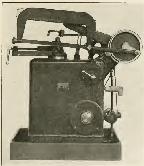
Portable Self-Contained Power Hack Saw
