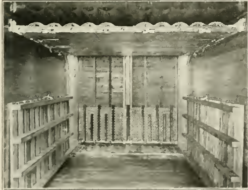
Bulkhead Sections and Floor Racks Raised to Permit Loading Entire Length of Car Body
