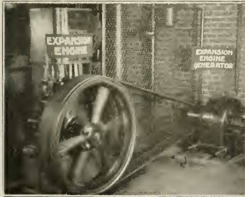
Fig. 5—Expansion Engine for Lowering Pressure and Temperature of Air
