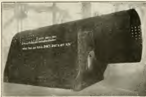
The Firebox Side Sheets and Crown Sheet and Combustion Chamber Are All in One Piece, the Throat Sheet Being Welded in as Shown by the Light Line
