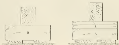
Lumber Bearing Built of Sound Salvaged Material
