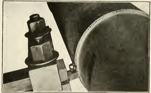
Fig. 3—Lathe Tool Just After Failure; Illustration Shows "Glaze" Produced On the Test Log
