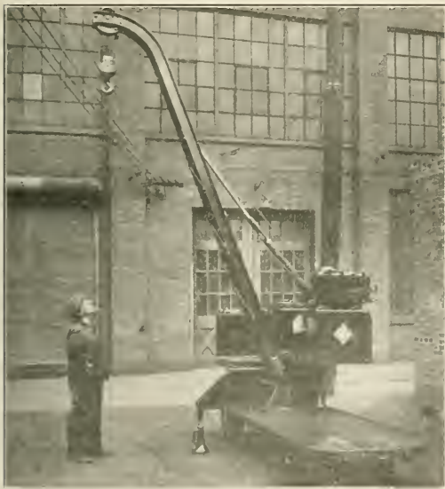
Fig. 1—Elwell-Parker Truck with 8-Ft. Outreach Power Crane
