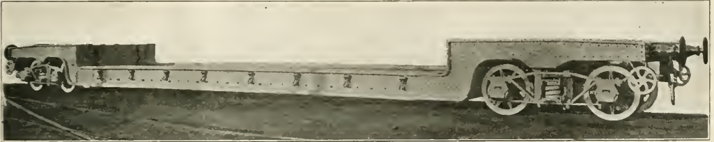
40 Ton Car with 34 Ft. 6 In. Well
