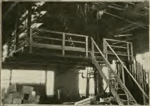
Fig. 7—Easily Accessible Storage Platform for Templates
