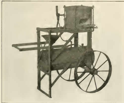
MacLeod Portable Suction-Type Rivet Forge
