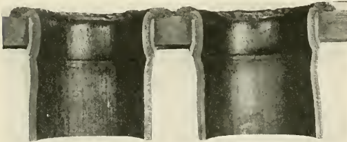
Fig. 1—Section of Tube Sheet with Charcoal Iron Boiler Tubes Welded in Place
