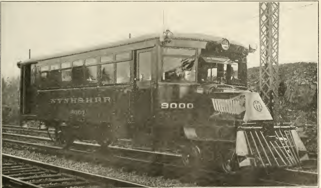
Mack Rail Car, Used in Local Passenger Service on the New Haven
