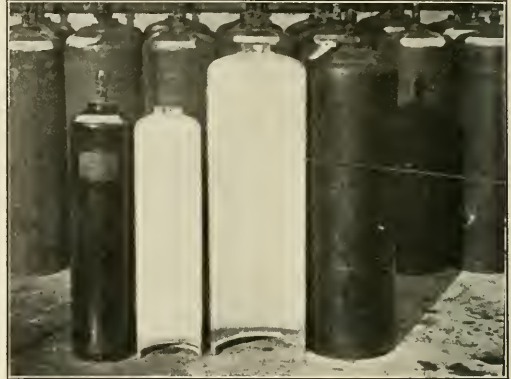
Fig. 4—Cross Section Through Acetylene Cylinders Showing Infusorial Earth Packing
