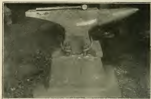
Durable Cast-Iron Anvil Block Used on the Chesapeake & Ohio
