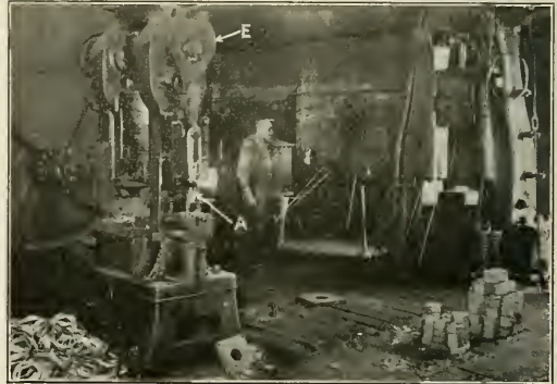
Fig. 11—Drop Hammer and Trimming Press Making Large Nuts
