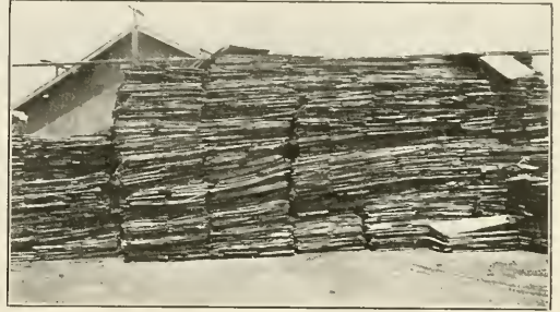
Defective Roof Sheets Formerly Used for Building Purposes or Sold for Scrap
