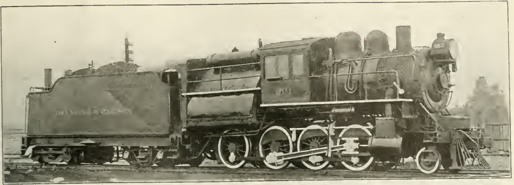
Superheated Consolidation Locomotive to Which the Tender Booster Has Been Applied
