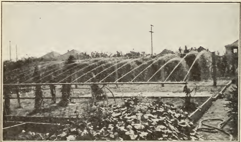
FIG. 8.—Portable spray equipment used in gardens about cold frames, hotbeds, etc. [Luther Burbank's gardens, Santa Rosa, Cal.]
