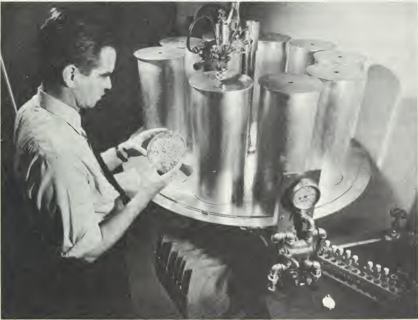
Counting the flies killed by an insecticide under test. The apparatus—aluminum drums on a turntable—was especially designed for these tests.
