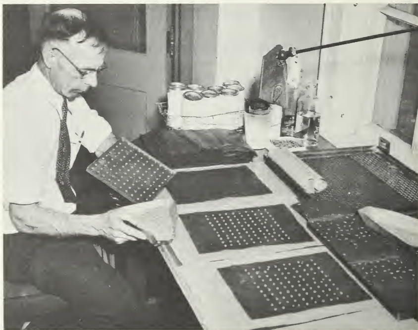
Preparing a sample of field pea seeds for a germination test. The tray in the seed technologist's left hand is a vacuum counter which automatically counts out the number of seeds desired.
