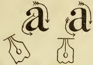
Position of pen and direction of lines in drawing Old Style (left) and Modern (right) that show the points of difference between the two styles
