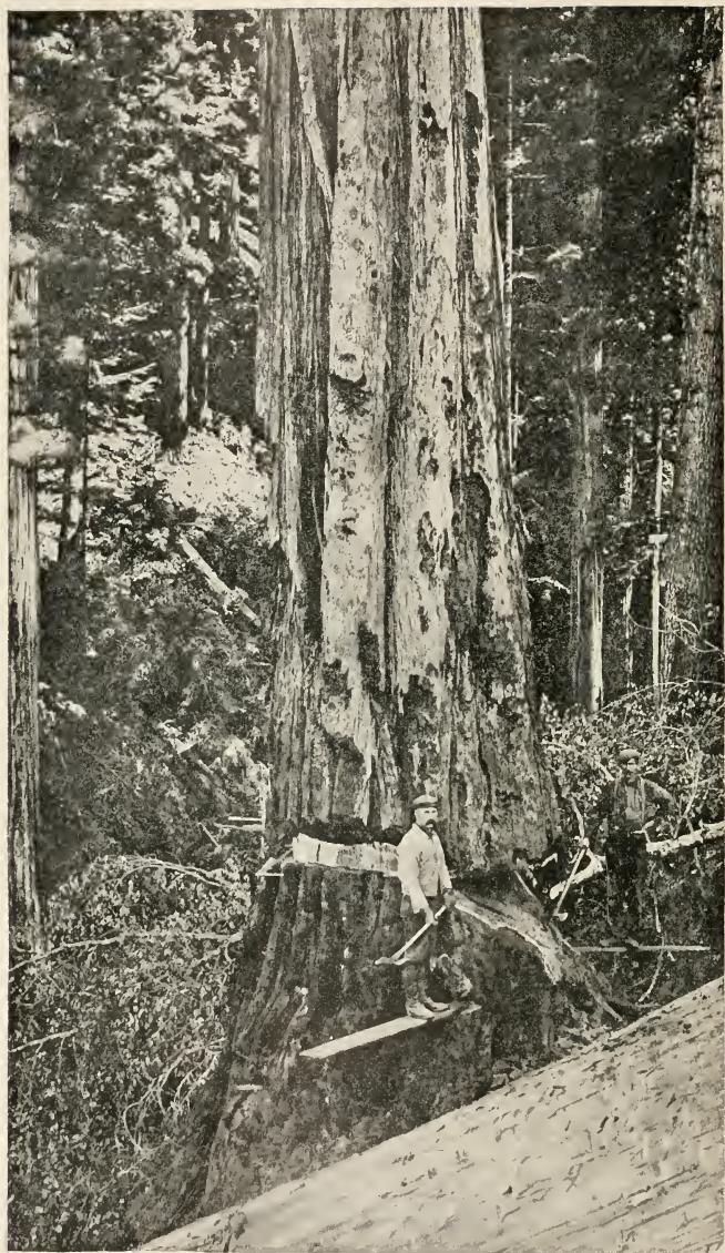
REDWOOD LOGGING. "FALLERS" MAKING THE UNDERCUT, CASPAR, MENDOCINO COUNTY, CALIFORNIA. AFTER THIS HAS BEEN DONE AND THE BARK CUT AWAY, A SAW IS USED. (SEE PAGE 300.)
