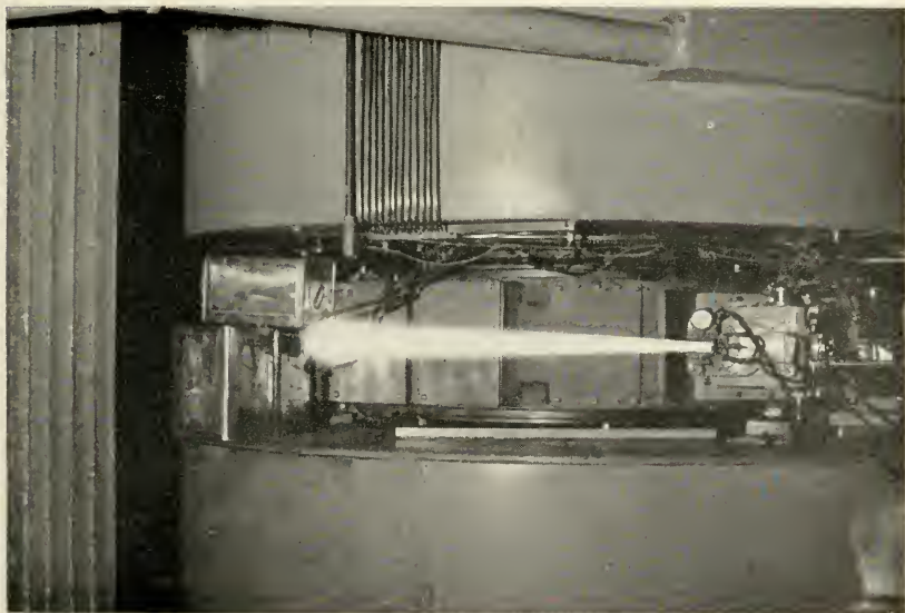
2. THE CYCLOTRON RELEASES A BEAM OF DEUTERONS. THE "ATOMIC BULLETS" OF TRANSMUTATION.
