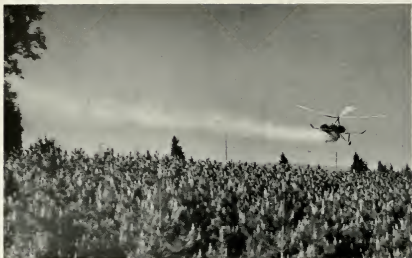
1. AUTOGIRO IN ACTION SPRAYING CONCENTRATED OIL-LEAD ARSENATE MIXTURE OVER RED PINE PLANTATION INFESTED WITH NEODIPRION SERTIFER.
