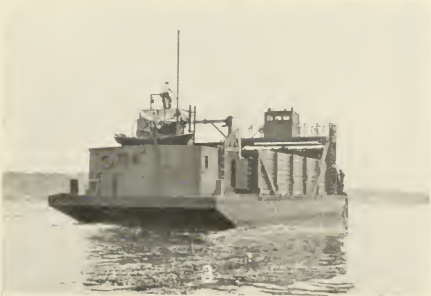
1. The giant kelp Macrocystis pyrifera in its natural habitat; 2 and 3, a power-driven barge harvesting kelp. Courtesy of the Keleo Company.
