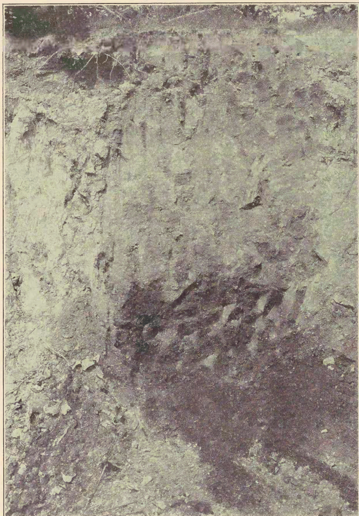
FIGURE 21.—Detail of the A horizon of Leonardtown silt loam, near Washington, D. C., showing lamination.
