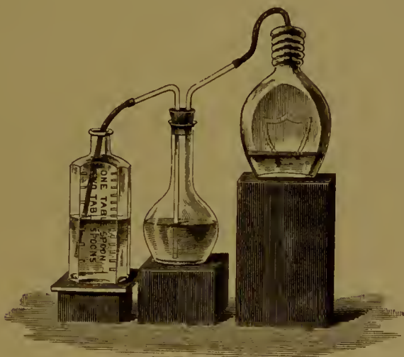
Fig. 3.—APPARATUS FOR ESTIMATING DIABETIC SUGAR BY FERMENTATION.
