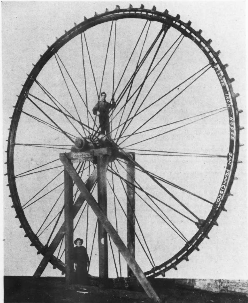
30-FT. DIAMETER IMPULSE WATER-WHEEL FOR A HEAD OF 775 FT.
