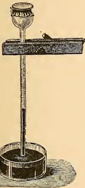
Apparatus to demonstrate lifting power of evaporation. (After Oels.)
