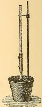
Apparatus for demonstration of root-pressure. (Detmer.)
