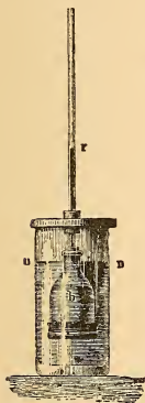
Osmometer. (Müller.) b , bulb of thistle-tube; D , level of liquid in cylinder; r , level of liquid in tube after a few hours' operation.
