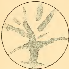
Marble plate corroded by roots. (Detmer.)
