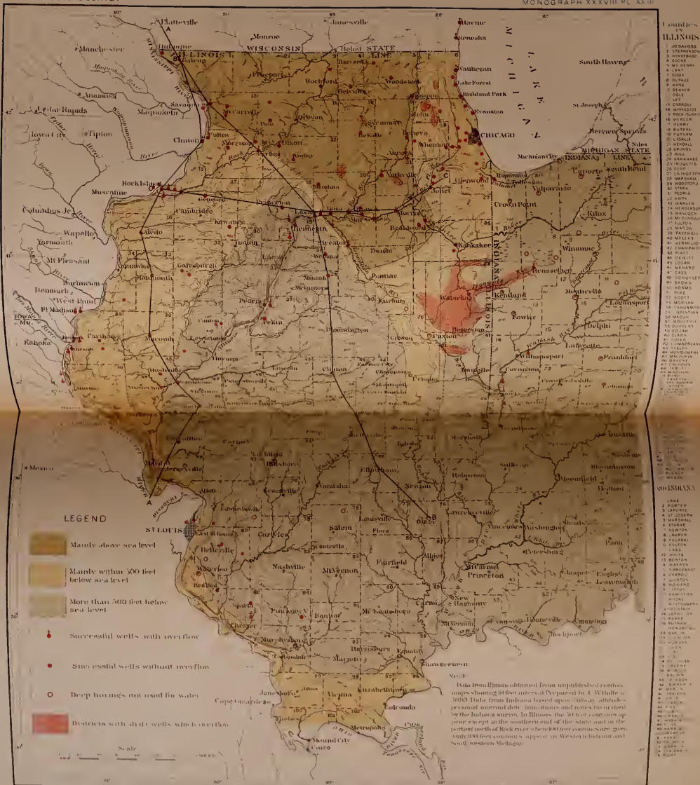
HYPSOGRAPHIC MAP OF THE ST. PETER SANDSTONE OF ILLINOIS AND WESTERN INDIANA Showing distribution of artesian wells and deep borings
