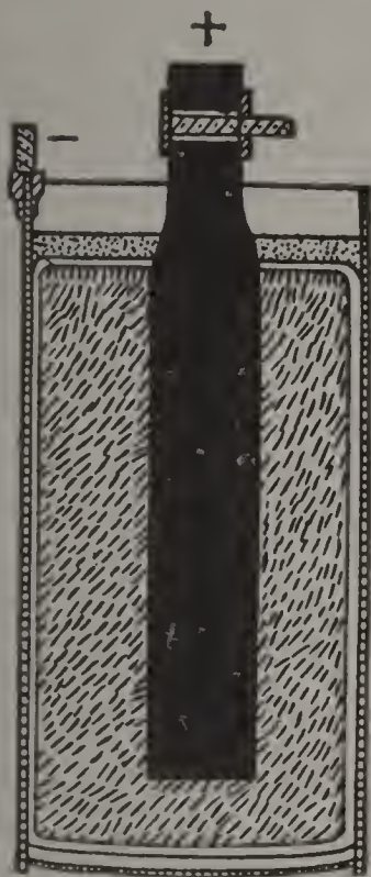
Fig. 31 Section Through Dry Cell
