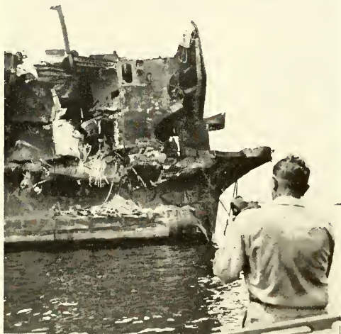
The light carrier INDEPENDENCE, located between 1000 feet and \frac{1}{2} mile from the projected Zeropoint, shows severe damage. Her 600 foot flight deck is broken in several places. Part of the deck planking has burned. Her four stacks have been demolished, and her antenna masts are bent or broken.
