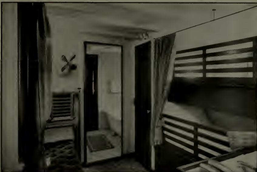
Children's nursery in the largest motor yacht afloat—a 154-footer. The picture shows one of the bathrooms, an electric fan run by current generated by an auxiliary lighting set, and a hot water radiator
