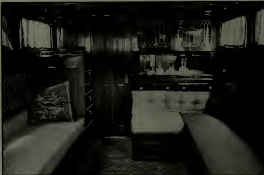
Main saloon of the Roslyn (54 feet), looking forward toward door to the galley. The two seats are of the extension type which make up into full width berths at night
