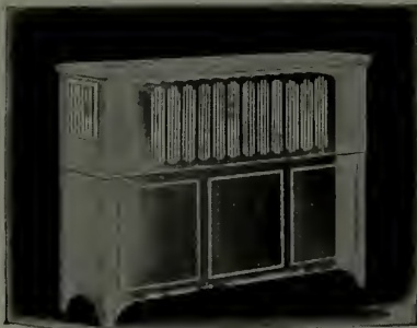
Phantom view of Ja-Nar' over radiator Air at room temperature passes over a sensitive but very simple and strong thermostat. This opens or closes the openings in the front, letting out or keeping in the heat and maintaining the temperature desired. The Ja-Nar' is perfectly insulated, and returns to the heating system any heat not needed.
