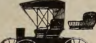
No. 117—Bike Wagon, with short wood caps on axles and full circle fifth wheel. Has 1 1/2-inch Kelly Cushion Tires. Price complete $65.50. As good as sells for $75 more.
