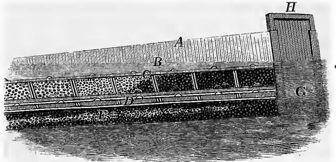
A. Top of Race. B. Water Level. C. Upper Screen, or Sieve. D. Under Screen. E. Bottom of Race. G. Supply Pond. H. Filtering Gate.
