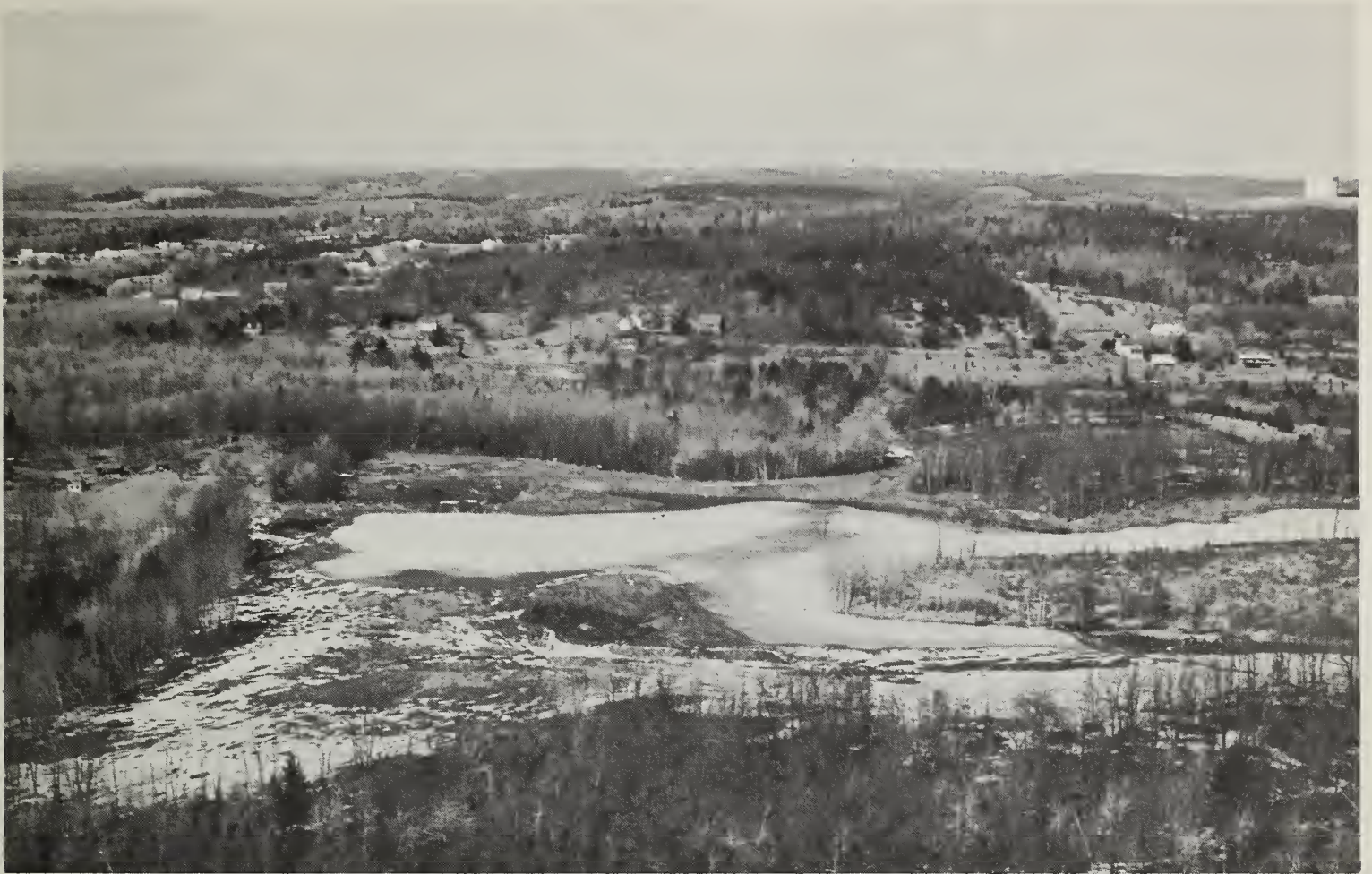
Westborough -- An aerial view of Cedar Swamp, north of the railroad, showing the "Equal Pondage Area" constructed to offset flood storage lost from industrial development. (W.R.C. photo)
