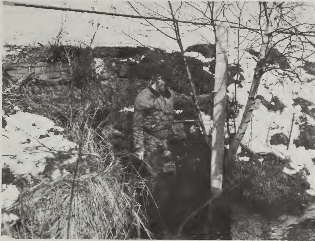
Westborough -- Staff gages were installed at key locations in Cedar Swamp to record fluctuations in water levels. This is location 7 shown on Plate 4. (SCS photo)
