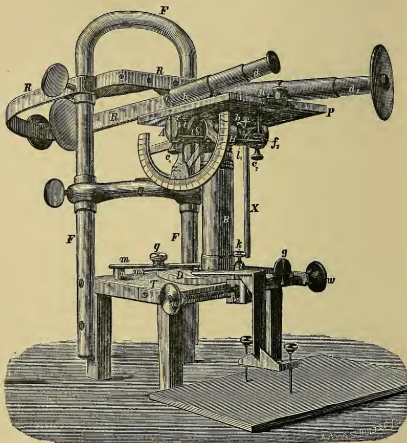
central point of the arc to  $90^\circ$  in either direction, whence the length of the radius can be calculated by appropriate formulæ given by the author.
