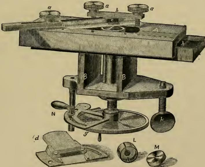
steel clamp and shoe *b* and *c*, with milled-head screws *a*. The carriage runs on a solid iron track *h* and *B*, which is held to a table by clamp screw *k*.
