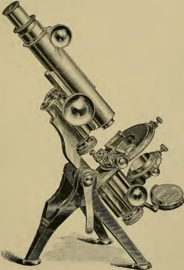
There is the usual rackwork coarse-adjustment. The fine-adjustment is a Campbell differential screw. This fine-adjustment, while being very strong, works with great smoothness and delicacy. It is claimed that the differential screw solves the difficulty which has always
