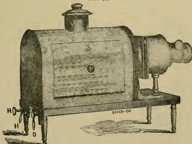
the condensing lens parallel with its axis; adjust Microscope or stereopticon lens; place the object on the stage, or, if a transparency, in front of the condenser, and a well-defined image is seen on the screen. To use the optical parts of the instrument just described with artificial
