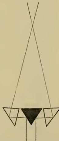
*Goltzsch's second Binocular Microscope.*†—We have already described ‡ Herr H. Goltzsch's first binocular Microscope, one of the features of which was the use of small telescopes for eye-pieces. He subsequently announced an improvement, by which the inconvenient vertical stage is dispensed with.
