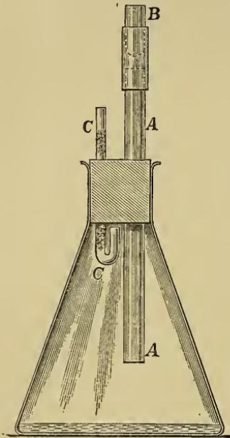
Ten cem. of Koch's pepton-gelatin are introduced into the flask, and the stopper tied on with copper wire. The flask is then steamed for an hour at  $100^{\circ}$  C., and on cooling, an even layer of gelatin is distributed over the bottom.
