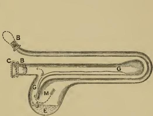
orifices are replugged, and then the gelatin melted by the aid of very gentle heat. The instrument is then placed in the horizontal position, fig. 117, so that the water and gelatin mix together in the bulb M. When thoroughly mixed, the fluid is dispersed over plates for the cultivation of this organism. The removal of the gelatin mixture is easily effected through the opening B.
