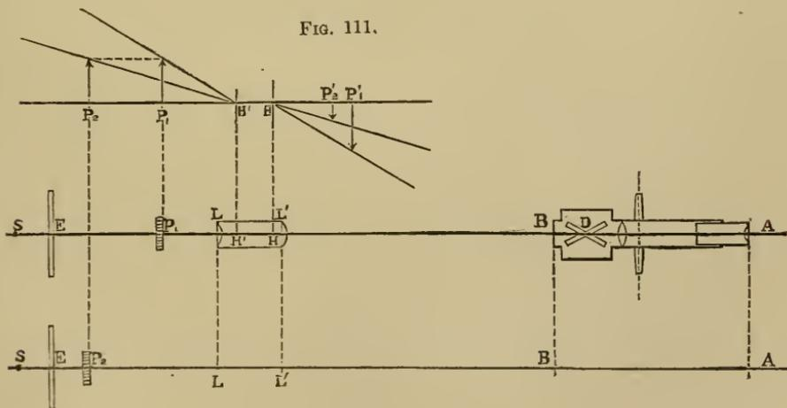
dition, therefore, should be as large as possible, so that the image might form as near as possible to the eye. If, on the other hand,  $d_0 > f$ ,  $1 - d_0 F$  is negative, and to augment the amplifying power  $L'$  must diminish, i. e.  $l'$ , the distance of accommodation, must be as large as possible. The most advantageous case is that of a hyperpresbytic eye, in which case  $L'$  is negative. For the Microscope the conditions are inverse.
