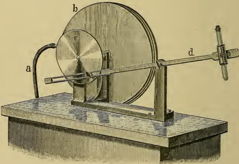
through the tube *a*, and removed by a similar tube not shown in the illustration. The water-wheel drives a circular metal disc *c*, in which, in one radius, is a series of holes. Into any of these holes is fixed a screw which connects the forked end of a long lever *d* to the apparatus. At the other end of the long piece *d* is a clamp for holding the test-tube, which is plugged when the apparatus is in motion.
