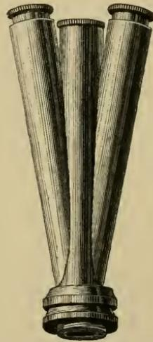
*Holmes's Isophotal Binocular Microscope.*—This is shown in fig. 76. The optical principle of the instrument was described at p. 870 of Vol. III. (1880). A peculiarity of the mechanical arrangement is that the tubes are made to rock from side to side on a socket. The object
