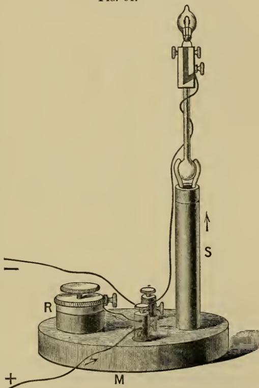
consists of a copper plate, 20 cm. by 10 cm., supporting at one end the lamp as described above, and on the rest of its length a horizontal complementary rheostat. The latter consists of a long tube of serpentine inclosing 120 discs of graphite, and gives a range of resistance from  $1/4$  ohm to 1000 ohms.
