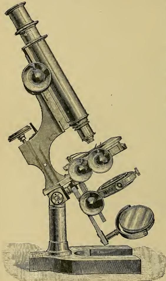
attached; it can be clamped by the screw in front. The substage has centering movements, rack-and-pinion coarse adjustment, and differential-screw fine-adjustment, admitting of wide-angled condensers being easily focused. The usual plane and concave mirrors on a double-jointed arm are carried on an adjustable hinged tail-piece.
