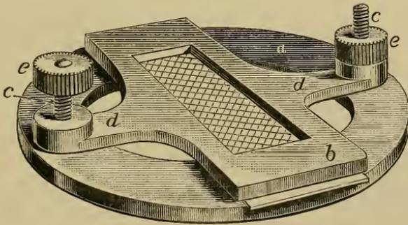
lies the oblong frame *b*. From the long sides of *b* two pieces *d d* extend, and end in rounded extremities, through which pass two screws *c c*. These connect the two movable parts, and when the screw-head *e* is turned down, these two parts are firmly fixed together.
