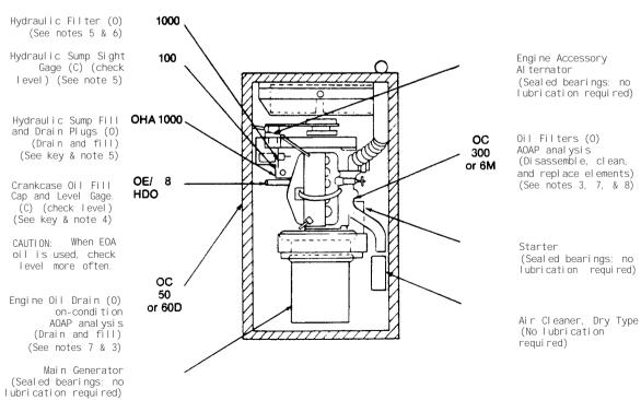
\*The time specified is the time required to perform all services at the particular interval (On-condition or hard time).
