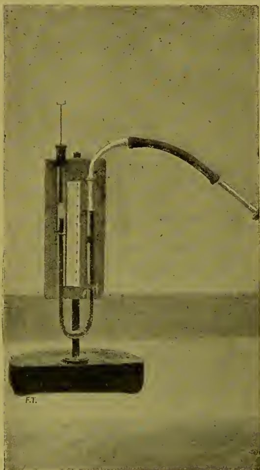
FIG. 7.—Mercurial manometer for the registration of the force of the respiratory movements.
