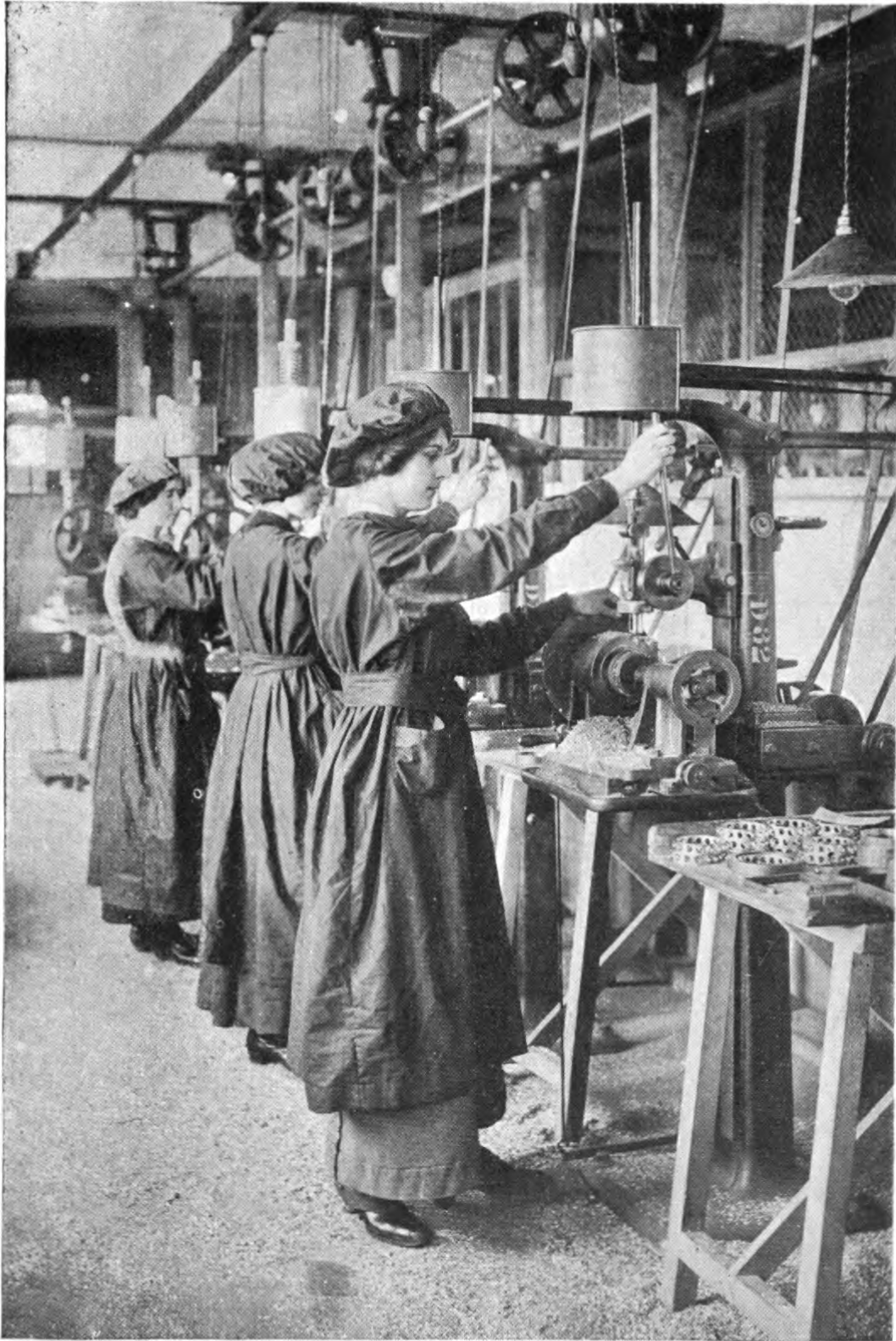
View of girls operating drilling machines on ball bearings.
