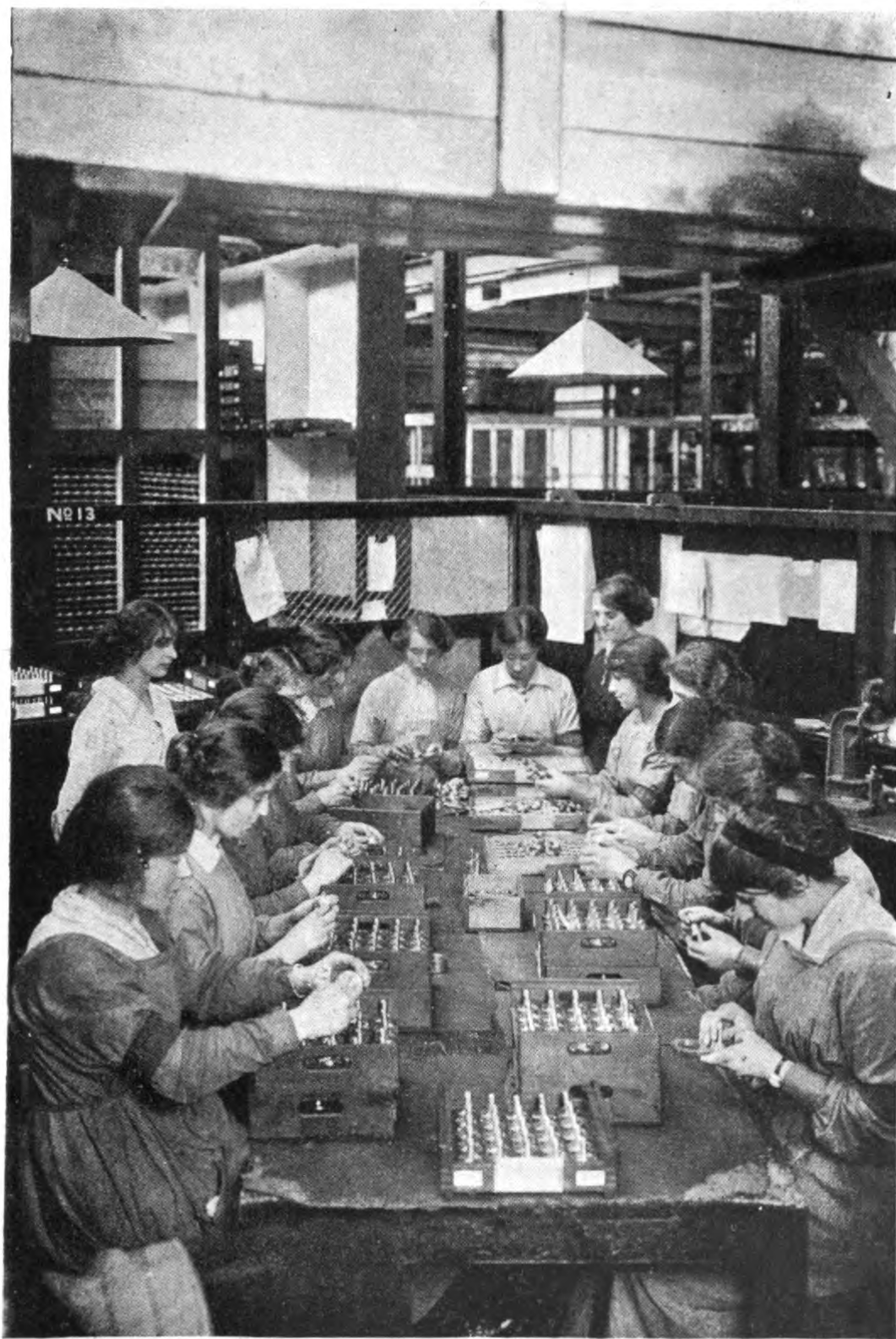
Inspecting and gauging fuse bodies.
