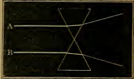
FIG. 10.—Divergence of rays by prisms.
