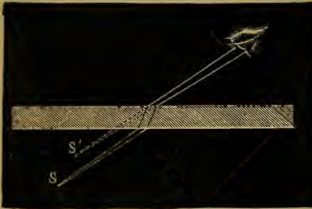
FIG. 27.—Apparent displacement of a luminous point by a parallel plate. (Deschanel.)
