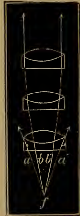
FIG. 26.—Angle of aperture of the objective. ( Dip-pel. )
