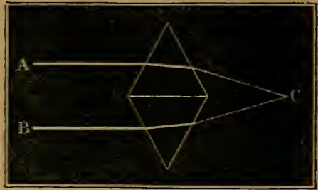
FIG. 9.—Convergence of rays by prisms.
