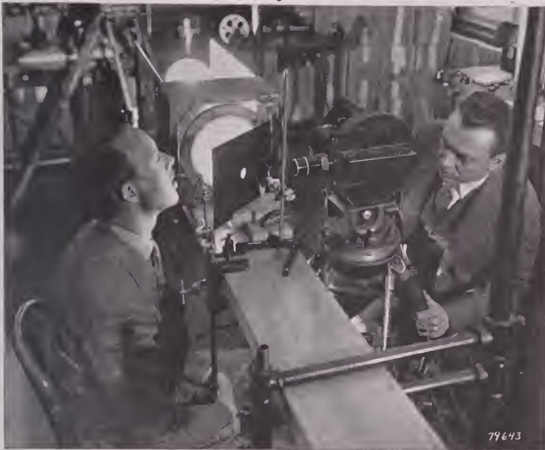
Fig. 2. The Fastax camera set up for photographing the vocal cords. The light beam is directed by the large mirror into the mouth, and then directed down the throat to the larynx by a small laryngeal mirror held near the soft palate. The camera shoots through the hole in the center of the large mirror and down onto the vocal cords by means of the laryngeal mirror.
