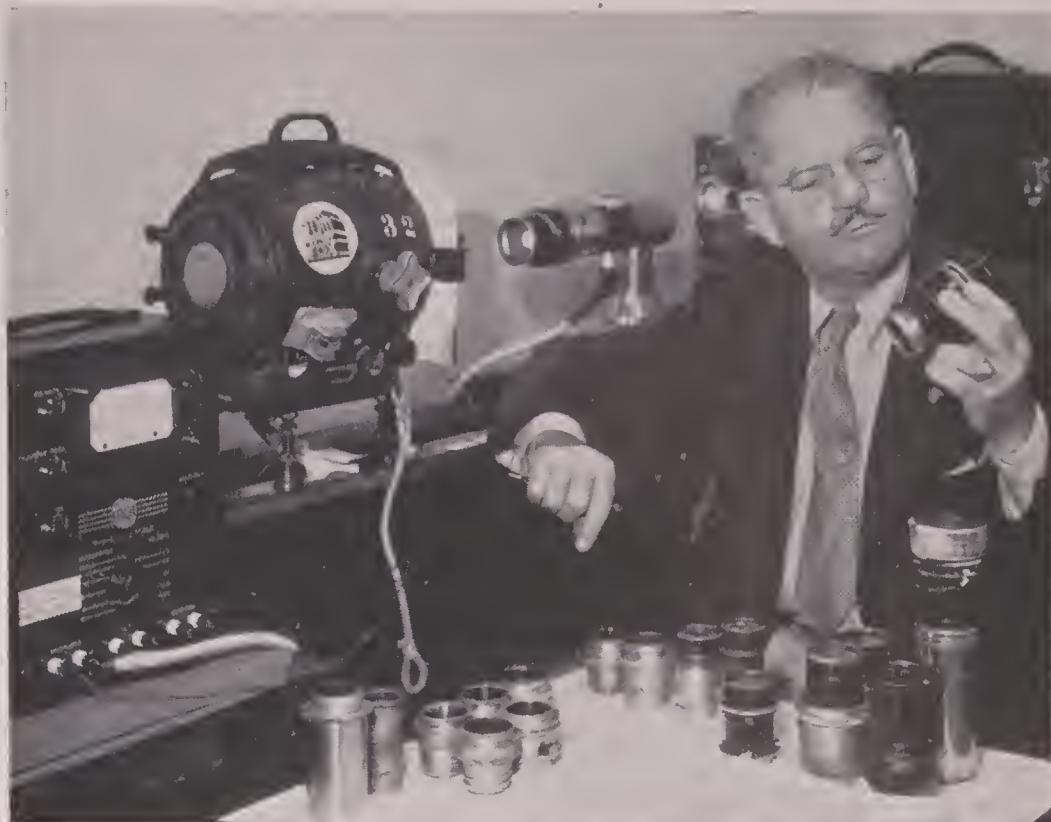
The author testing lens-transmission during his initial experiments. The equipment now in use has been made more compact, and a simple light-box has replaced the "baby keg" as a light-source.
