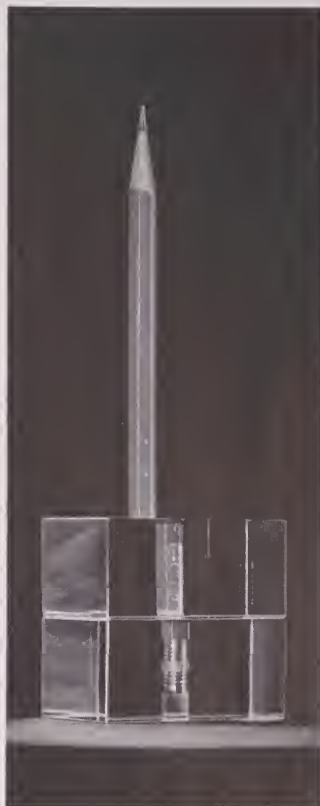
POSITION OF PENCIL'S IMAGE shows that Kodak's new glass (below) has greater light-bending power than old-type optical glass (above). Both have the same dispersion.
