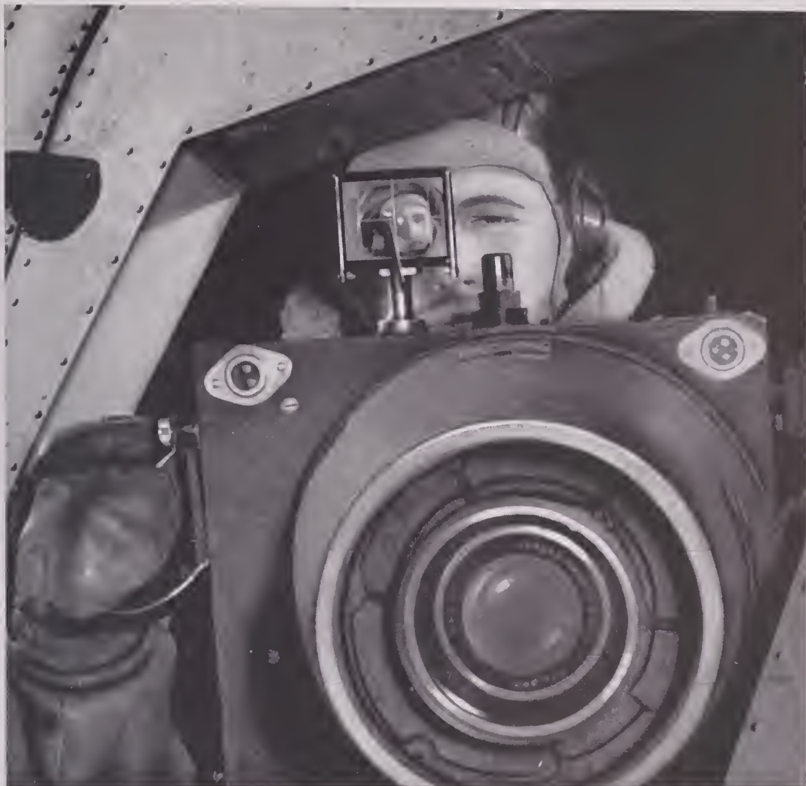
AIRPLANES MADE TO FLY FASTER and at greater heights present new problems to lens designers. Kodak's new glass, with a much higher refractive index (light-bending ability) than previously available in optical glass of the same dispersion, is now being applied to aerial lenses and is partly responsible for the effectiveness of our aerial photography. The new lens has twice the speed of the fastest lens previously used by our Army Air Force.
