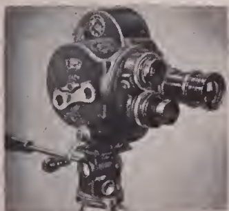
→ EYEMO MODELS P AND Q . . . These are similar to Models N and O, respectively, except that P and Q are equipped for alternate, optional use with electric motor and external film magazines. External film magazines extend maximum scene length from 55 to 400 feet. Offset finder eyepiece prevents interference.
