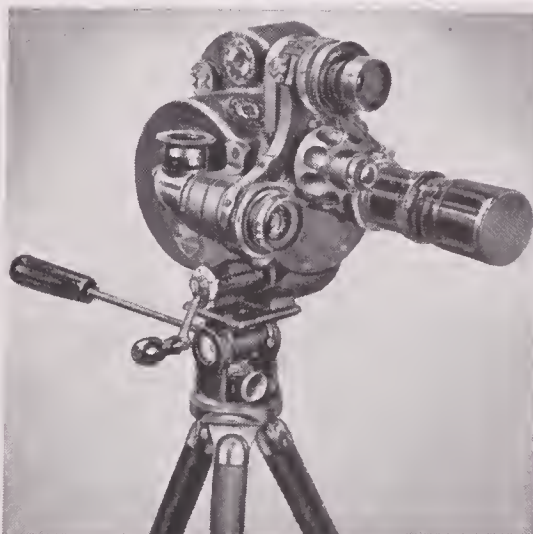
EYEMO MODELS N AND O . . . Three-arm offset turret permits broader choice of lenses. Turret lock is particularly appreciated with long, heavy lenses. Visual, prismatic focuser with magnifier. Model N has speeds of 4, 8, 12, 16, 24, and 32 f.p.s.; Model O has speeds of 8, 12, 16, 24, 32, and 48 f.p.s.
