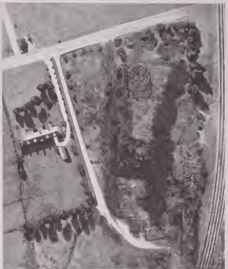
NOW YOU DON'T. With camouflage materials—false structures, netting, cloth streamers, paint, and artificial trees—the experts have fooled the camera, and the bombardier. To the aerial camera loaded with panchromatic film, even the marks of erosion on the slope by the railroad track have disappeared.
