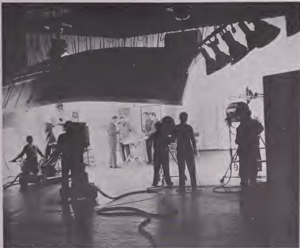
Telecasting a demonstration of Army Training Film production. The uppermost lighting units are 3 kw. mercury vapors. Next, the main bank of fluorescents rated at 7 kw. but actually the equivalent of 21 kw. due to greater sensitivity of the "like" to color temperatures approaching daylight. Overhead incandescents are 1000-Watt units totaling 5 kw. Spotlights are 5 kw. Total wattage on the set is 24 kw. Lens apertures, f:4.5. Iconoscope sensitivity equivalent to Weston 50.
