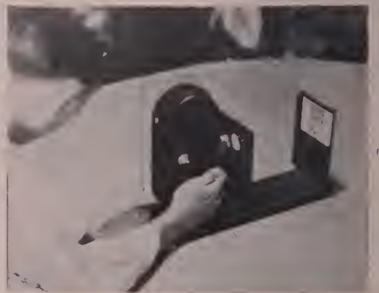
Top, a flat developing rack fits in standard size tray, and holds 25 feet of 16 or double 8mm. film. Next, the film is wound spirally around the rack. Adjoining film loops should be kept from overlapping by pins or grooves. Third from top: a contact print is made by threading the two films in the camera, emulsion to emulsion, with the shiny side of the raw film facing back of camera. Bottom, making titles by straight development.
