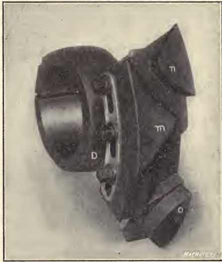
Fig. 10. Adjustable Cam for Controlling Operation of Chuck
