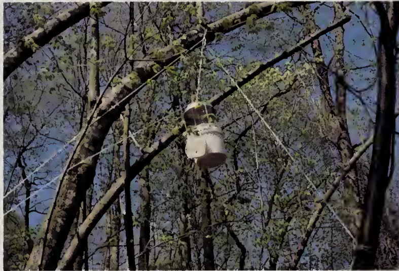
Figure 7-2. Blacklight trap used to collect nocturnal insects, especially moths, Fernow Experimental Forest.
