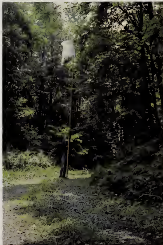
Figure 7-2. Blacklight trap used to collect nocturnal insects, especially moths, Fernow Experimental Forest.
