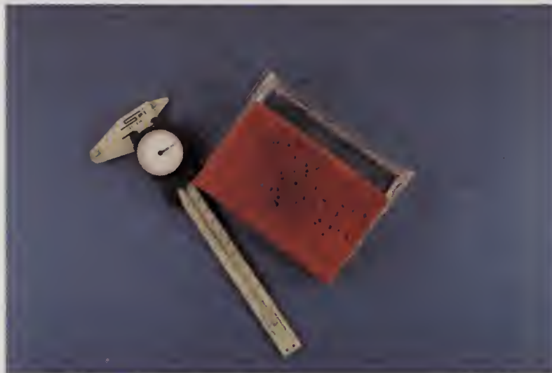
Figure 3-3. A device used to measure snout-vent-length of salamanders.
