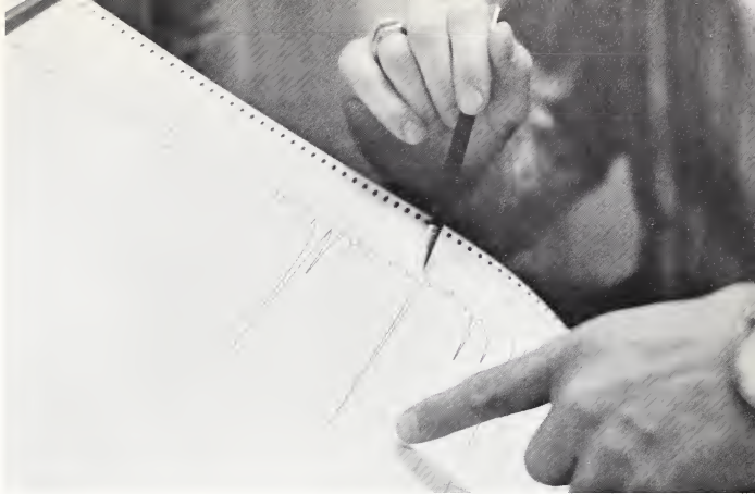
▲ This chromatograph printout indicates the amount of terpene compounds in the mixture
