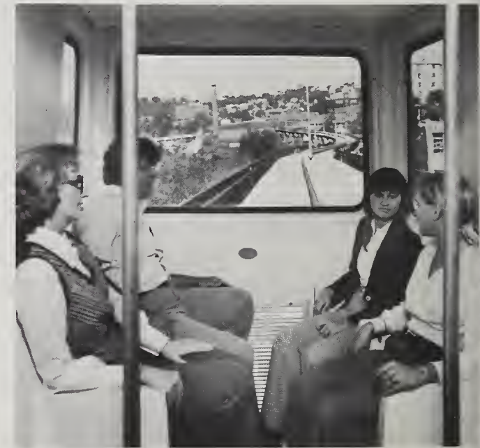
The Morgantown PRT vehicle carries up to 21 passengers, both seated and standing.
