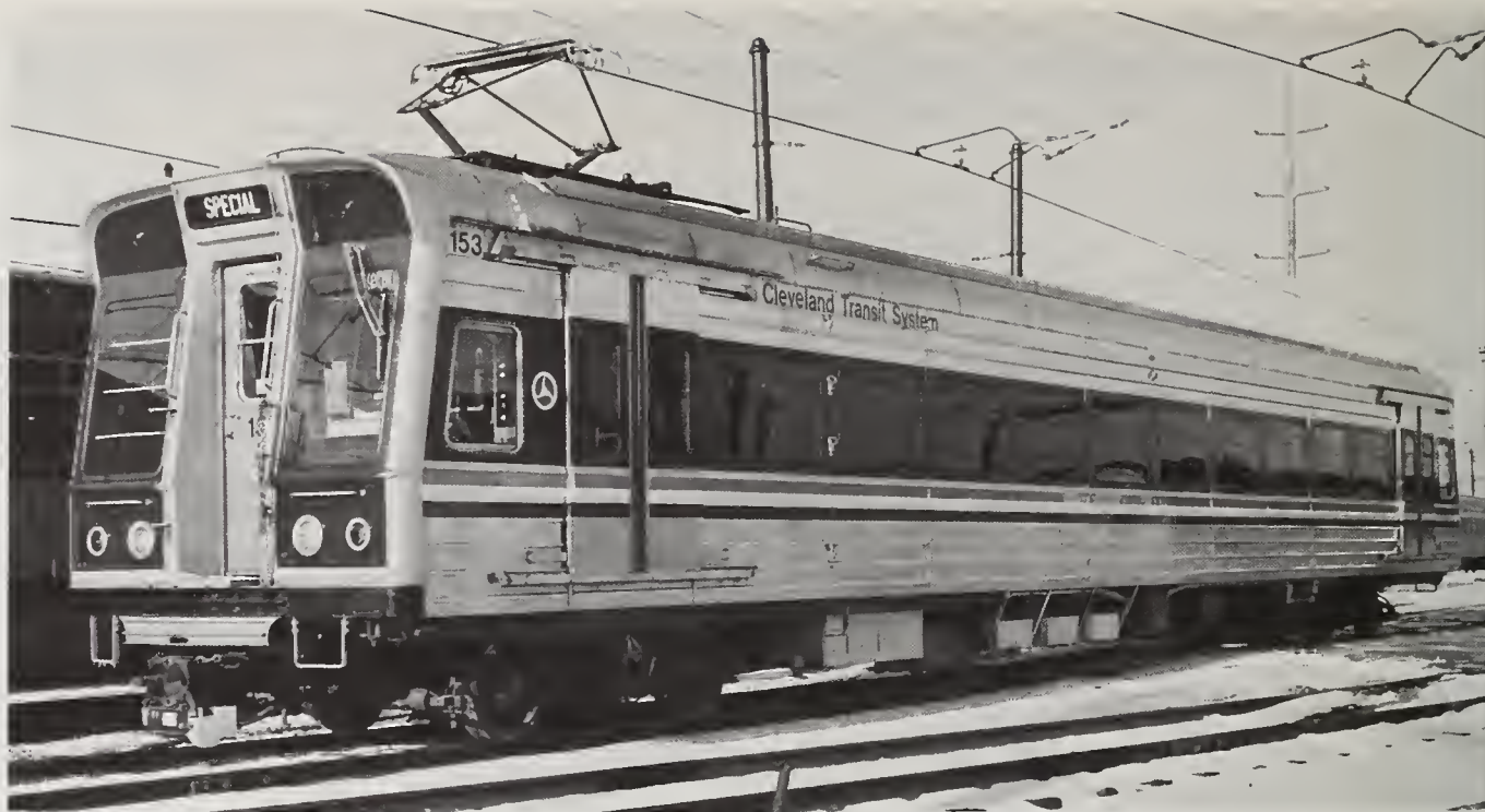
Three Cleveland Transit System "Airporter" cars were equipped with AC propulsion and control systems to test smoother acceleration/deceleration and power regeneration during the braking cycle.
