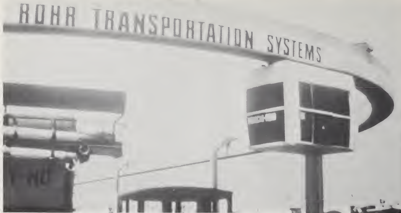
The Rohr Monocab system uses a suspended monorail and electromagnetic propulsion.
