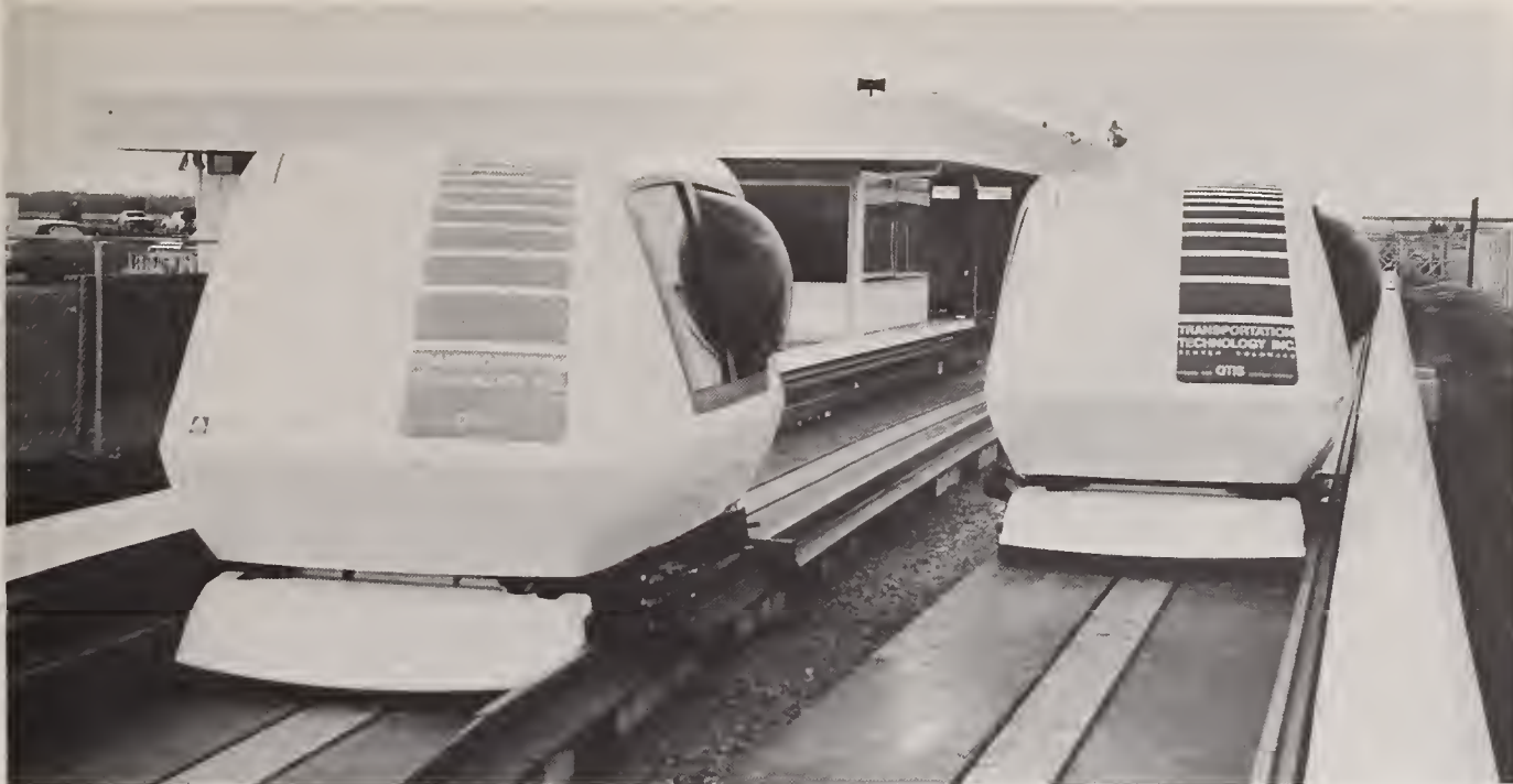
The Transportation Technology Air Cushion Vehicle was first demonstrated at Transpo 72 and then was evaluated in extended use at Dulles Airport outside Washington, D.C.
