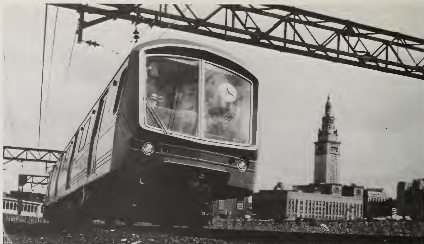
The State-of-the-Art Car (SOAC) demonstrated the latest in existing rapid rail technology.
