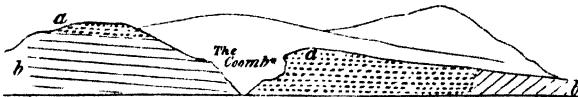
Fault coinciding with the Coomb, in the Cliff-hill near Lewes. Mantell. a. Chalk with flints. b. Lower chalk.
