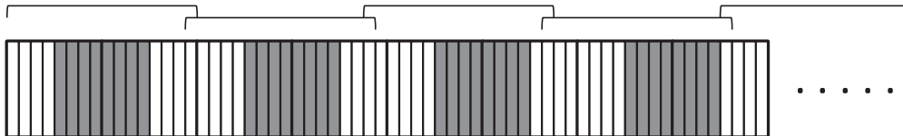
Figure 3.11: Best case layout example. The best case target data layout is when there is exactly one target block per transaction block. The target data are spread out across as many transaction blocks as possible.
