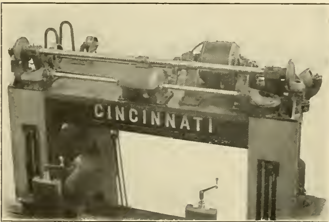
Motor Drive for the Rapid Power Traverse and for Feeding the Heads; Also for Raising the Crossrail
