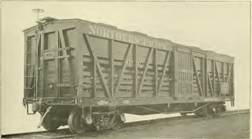
Stock Car of 80,000 lb. Capacity for the Northern Pacific
