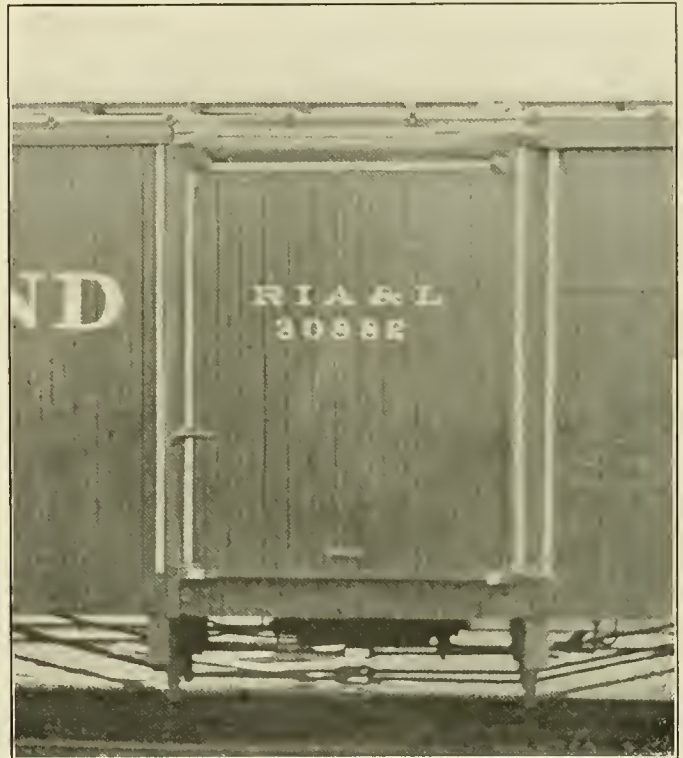
Car with Strips Applied for Flour Shipments
