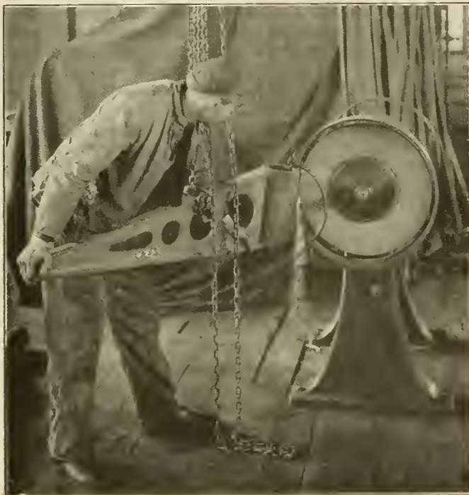
Hood Protection for Wheel When Snagging Heavy Castings by Aid of Chain Hoist
