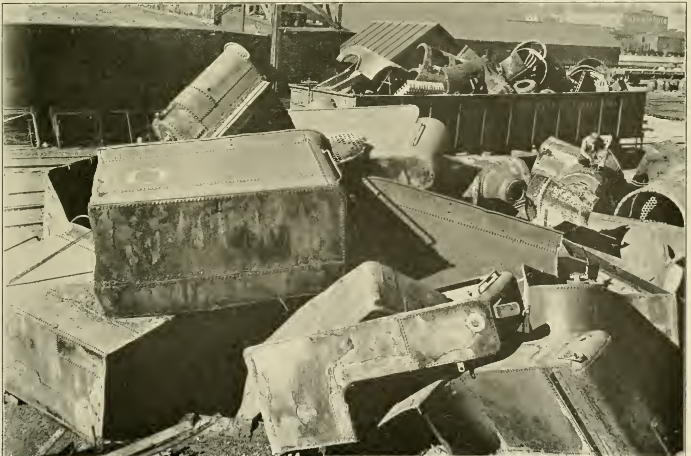
Old Locomotive Tanks Which Have Been Cut to Sizes Convenient for Handling.
