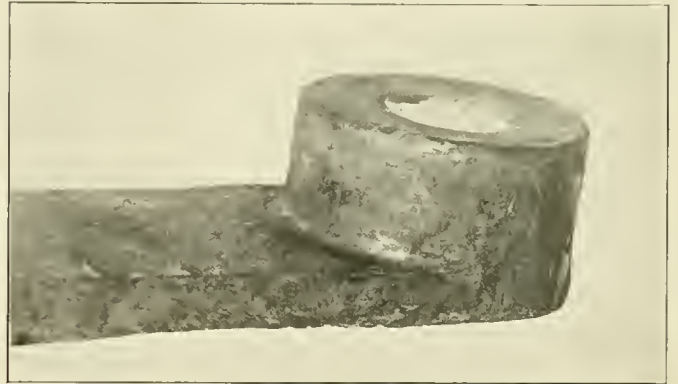
Fig. 2—Ash Pan Lever Made with the Dies Shown in Fig. 1
