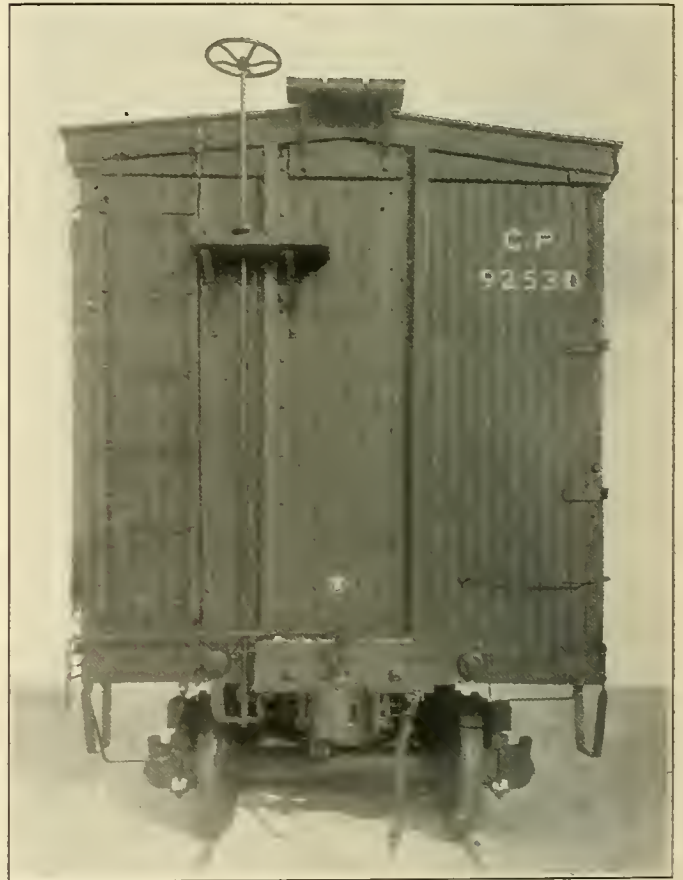
The Ends of Wooden Box Cars Are Reinforced with Z-Bar Posts Bolted Through the New Inside Lining
