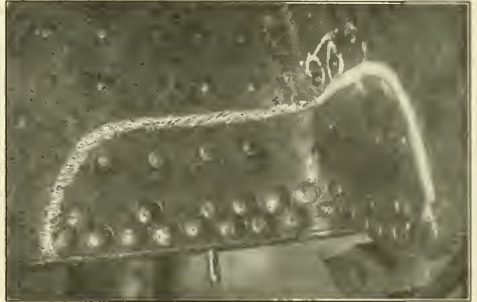
Piece Welded in the Corner of a Firebox
