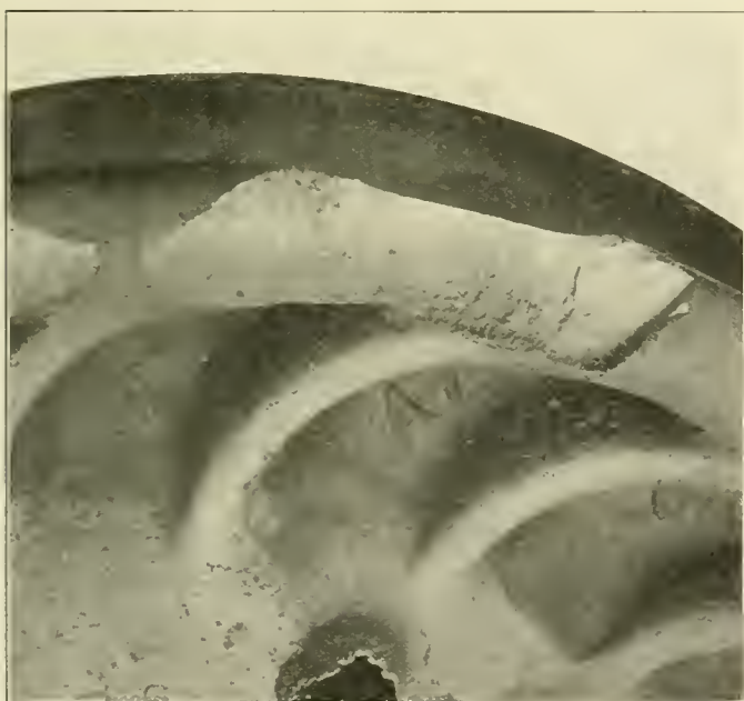
Fig. 2—Flange Broken with Hammer, Showing Direction of Fracture
