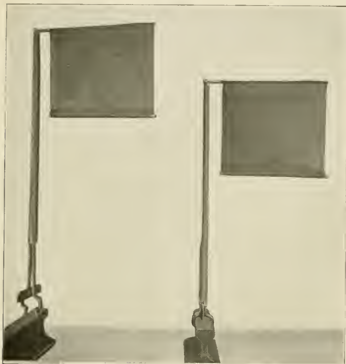
Blue Flag Holder Being Placed on a Rail, and After It Is in Position
