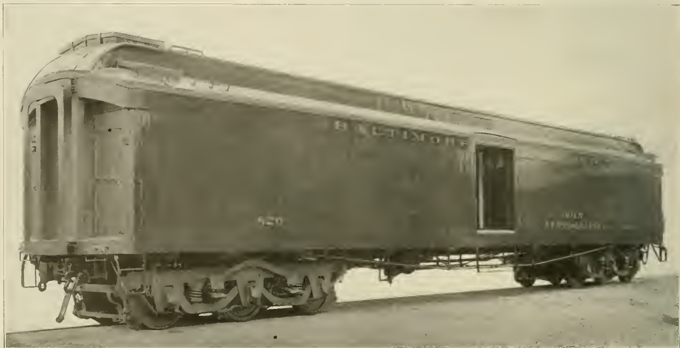
Refrigerator Car for Milk Traffic on the Baltimore & Ohio, Rebuilt from a Postal Car
