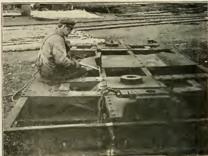
Cutting a Scrap Underframe, Thus Saving the Usable Parts and Securing a Higher Price for the Scrap
