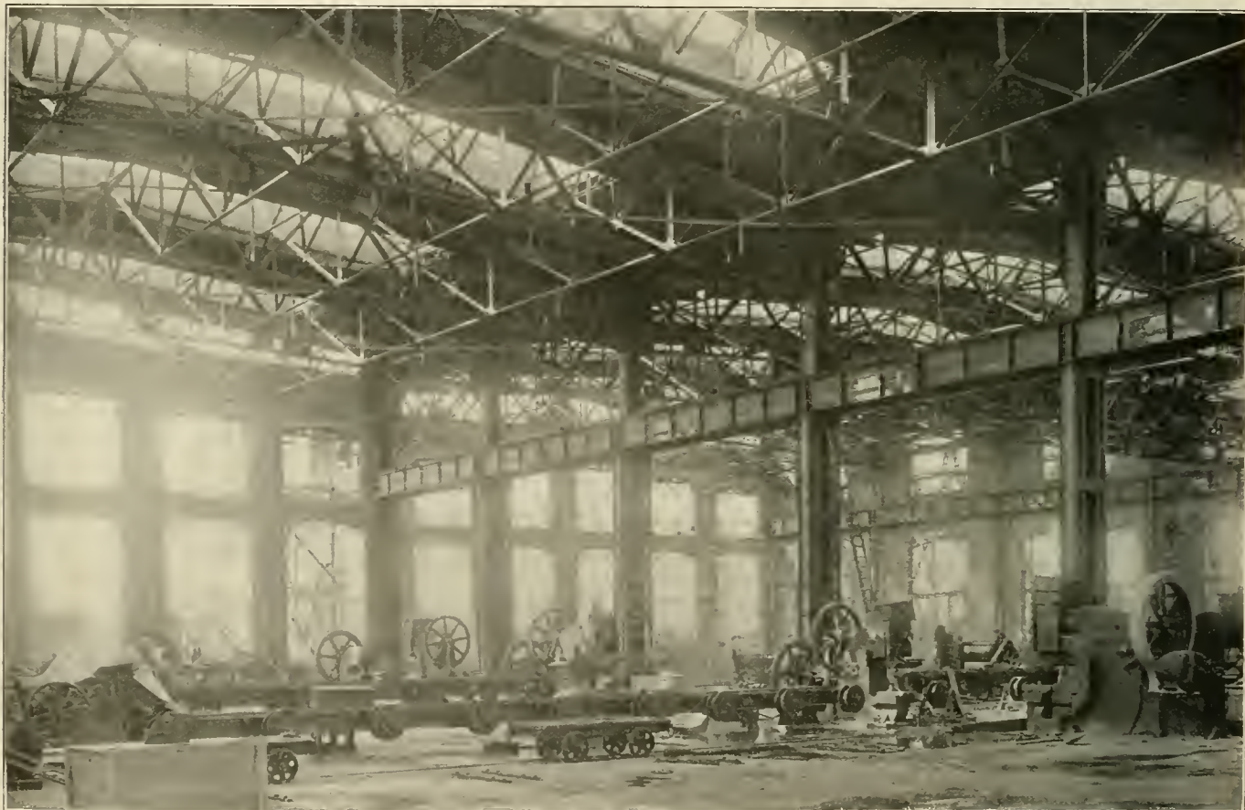
The Shop is Exceptionally Well Lighted; Spacing and Punching Machines are Shown in the Foreground
