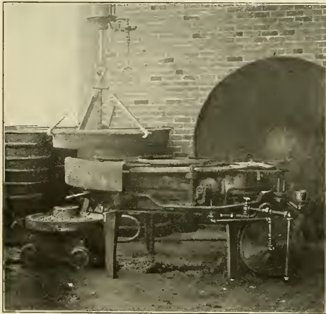
Fig. 16—Fuel Oil Heater Which is Placed Outside the Shop for Heating the Tires of Steel-Tired Wheels
