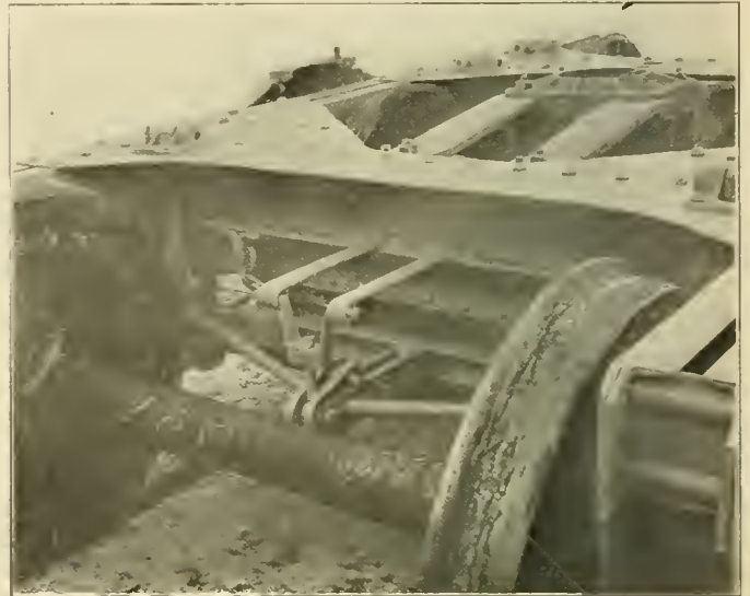
End View Showing the Brake Beam Adjuster and the Absence of the End Piece
