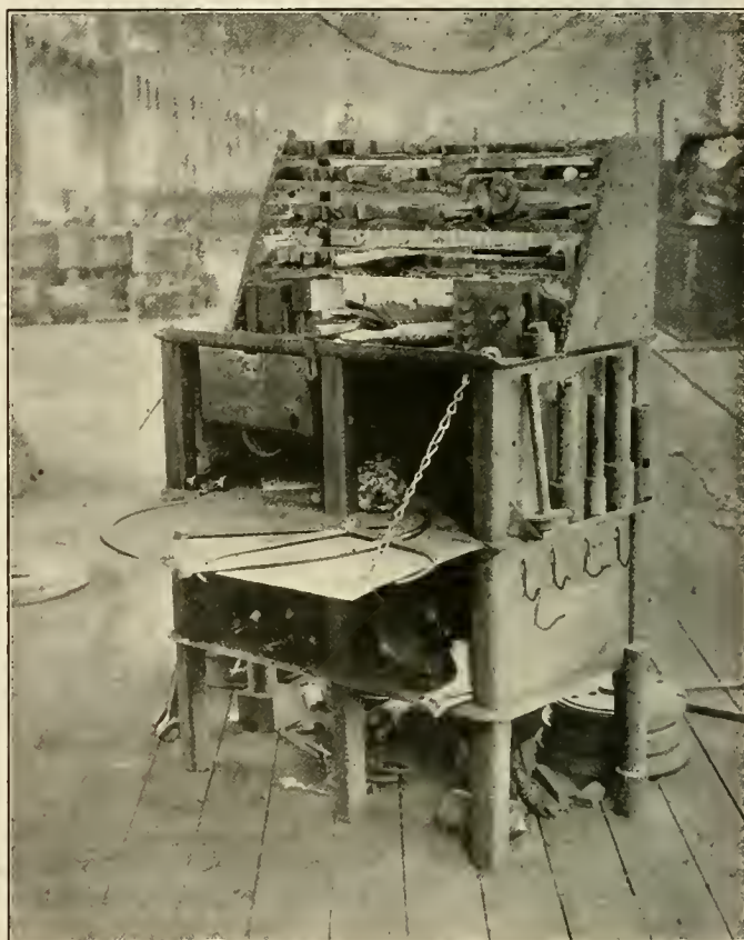
Steel Tool Cabinet for Use with Boring Mill
