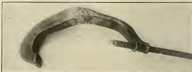
Clamp Welded by Oxy-Acetylene and Bent 45 Deg. Without Rupture
