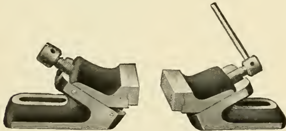
Divided Vise for Clamping Work on Machine Tools
