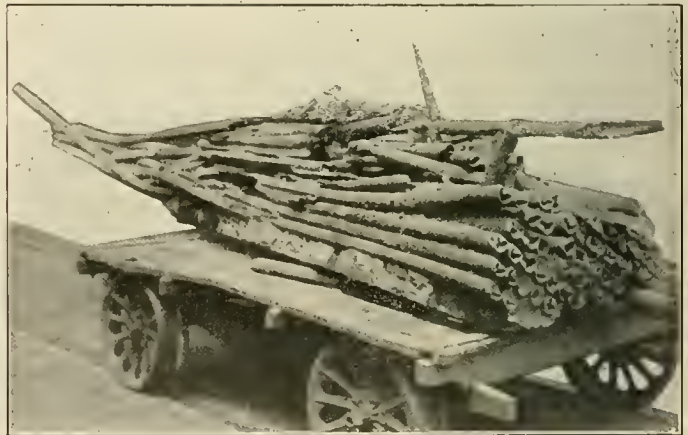
Fig. 6—Mass of Tubes and Solid Matter Taken from Bottom of Boiler Just Back of Injector Checks
