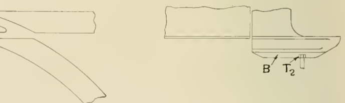
Fig. 3—Section Through Truck Side Frames at the Lower Flange of the Track I-Beam, Showing a Right-Hand Switch
