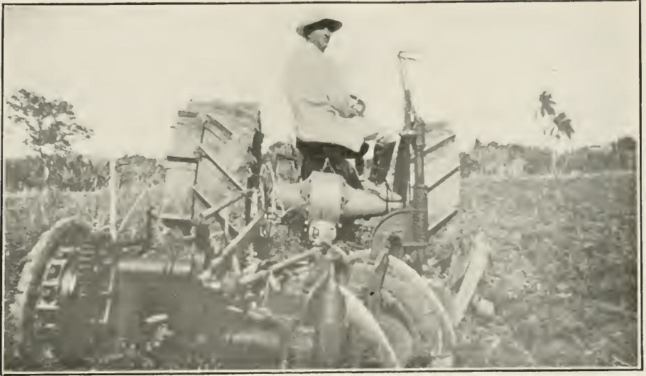
"Fordson" tractor hauling Oliver two-disc plow at Campo Florida, Cuba. (Courtesy of Mr. Martial Facio, Havana.)
