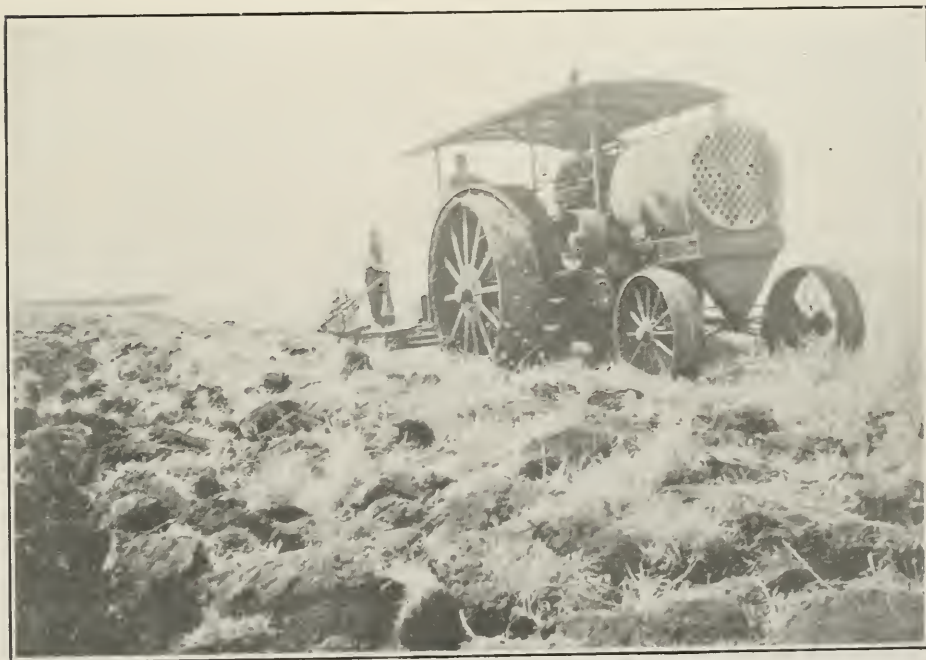
"Twin-City" 40 H. P. tractor hauling eight plows. (Courtesy of J. Z. Horter Co., Havana.)
