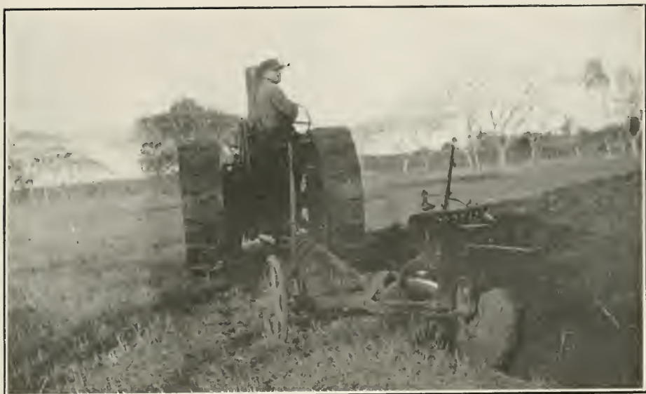
"Mogul" tractor 8 H. P. hauling two-disc plow. (Courtesy of J. Z. Horter Co., Havana.)
