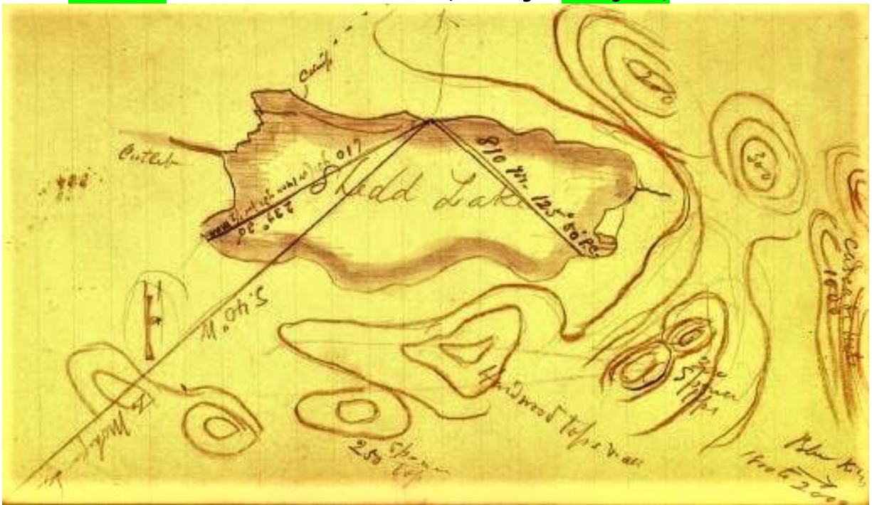
Shedd Lake Sketch with Lake Measurements, Heading to Mohegan L., Altitude Labels
