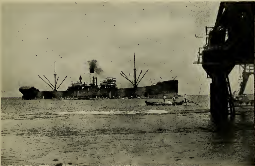
Nauru Island. Shipping phosphate in bulk from Nauru Island. The phosphate has to be lightered off in surf-boats—over 1000 tons can be shipped in 9 hours. The steamer is lying in 150 fathoms of water.
