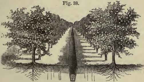
An under-drain between the rows.
