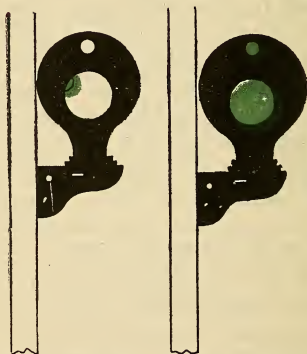
FIG. 117B. THE DISC TYPE OF SEMAPHORE.
