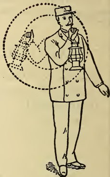
BACK —Swung vertically in a circle across the track.
