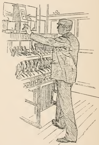
Signal Box, with Electrically-operated Signals.
