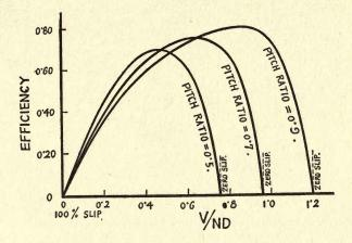
Fig. 56. Efficiency of three similar propellers with different pitch ratios.
