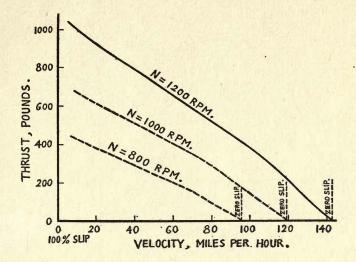
Fig. 51. Variation of thrust with velocity, for a particular propeller, when driven at constant speed. Pitch ratio 0.9, diameter 8'9".
