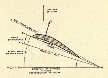
Fig. 60. Particular section of propeller blade at distance of r from center of shaft, showing the behavior of a propeller blade as an aerofoil, attacking the air at an angle of incidence i.
