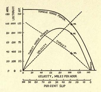
Fig. 52. Variation of thrust horse power with velocity for a particular propeller when driven at 1200 R. P. M. Dotted curves show thrust and velocity. The upper curve, reproduced from Fig. 47, shows torque horse power.
