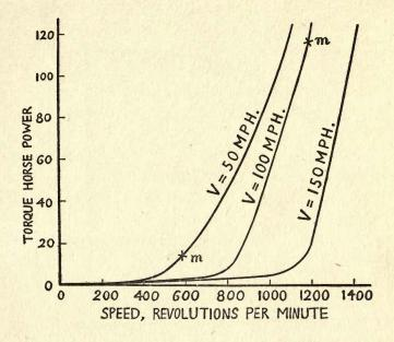
Fig. 46. Torque horse power required to drive a particular propeller at different speeds (revolutions per minute) when travelling through the air at 50, 100 and 150 M P H., at ground level. Propeller diameter, 8' 9"; pitch ratio, 0.9. Maximum propeller efficiency is at m.
