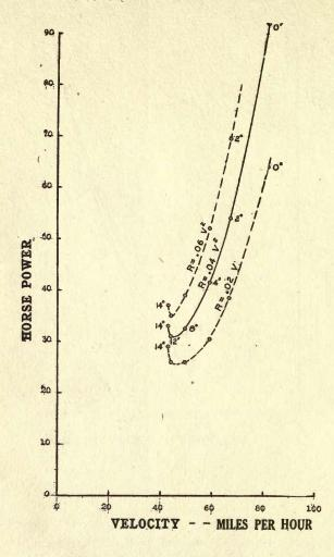
Fig. 43. Variation of required power with velocity. The three curves show effect of changing parasite resistance  $(R = 0.02 V^2, R = 0.04 V^2 \text{ and } R = 0.06 V^2)$ ; weight and loading constant (W = 2000 lbs.; W/S = 6).
