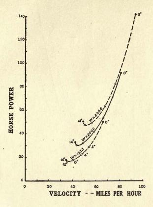
Fig. 42. Variation of required power with velocity. The three curves show effect of changing weight (W = 1333, 2000 and 2666 lbs.) and loading in proportion (W/S = 4, 6 and 8), wing-area being constant; parasite resistance =  $0.04V^2$ .
