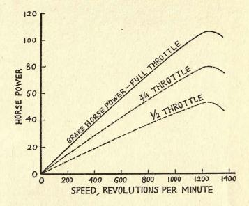
Fig. 44. Variation of brake horse power of a typical gas engine with speed. Dotted curves show reduction of power by throttle control.
