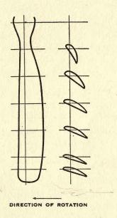
Fig. 59. Plan and section of propeller blade.
