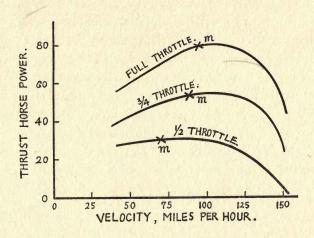
Fig. 58. Combined engine and propeller characteristic. Thrust horse power, or power available, for constant throttle; a particular propeller (pitch ratio 0.9, diameter 8'9") driven by a particular engine. Maximum efficiency at m. For engine curves, see Fig. 45.
