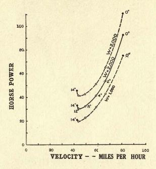
Fig. 40. Variation of required power with velocity. The three curves show effect of changing weight (W = 1000, 2000 and 3000 lbs.) when loading is kept constant (W/S = 6); parasite resistance = 0.04  $V^2$ .
