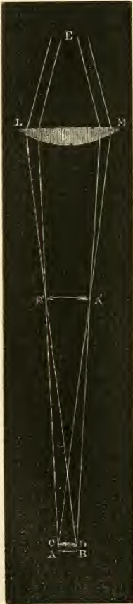
Diagram of simplest form of Compound Microscope.
