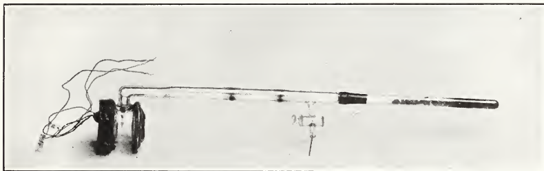
FIG. 36.— Device to record the heat of the stars and other radiation
