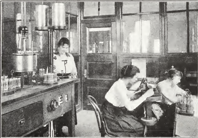
FIG. 26.—Group of bureau workers measuring the errors of clinical thermometers
