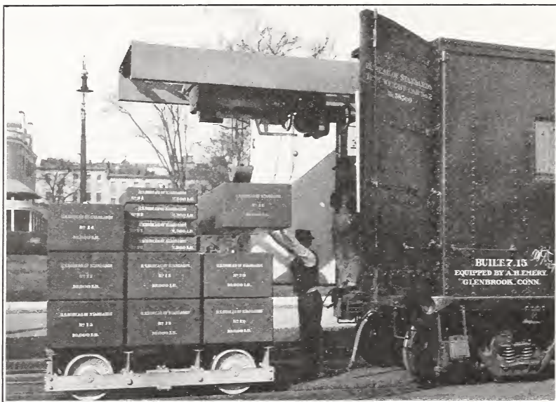
FIG. 24.—Track scale test car equipment
