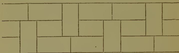
Fig. 16.—Hollow brick wall, 14 inches thick.
