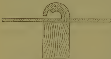
Fig. 30.—Section of roof tile.
