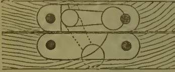
Fig. 44.—Plan of window-fastening.
