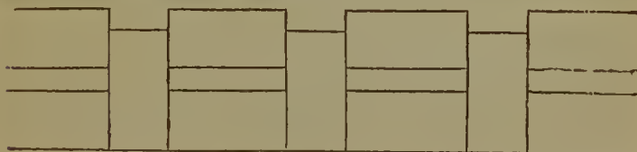
Fig. 14.—Loudon's hollow brick wall, 11 inches thick.
