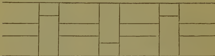
Fig. 15.—Hollow brick wall, 12 inches thick.
