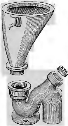
FIG. 79.—Stoneware hopper closet and trap.
