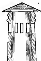
FIG. 2.—Section of a chimney-cap; the smoke passes out at slits in the masonry of the chimney. (Bosc.)
