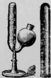
Fermentation-tube on left side ; ordinary tube on right side.
