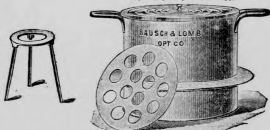
Iron tripod with water bath.
