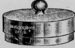
Moist chamber with a knob on the upper dish.
