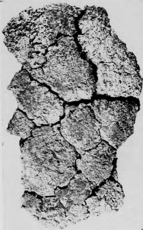
Gas retort coke from 33% Volatile matter and 12.8% Ash. "Coal Mixture" of 40% Chunghsing coking coal and 60% Tatung poorly coking coal 1/4" full size.
