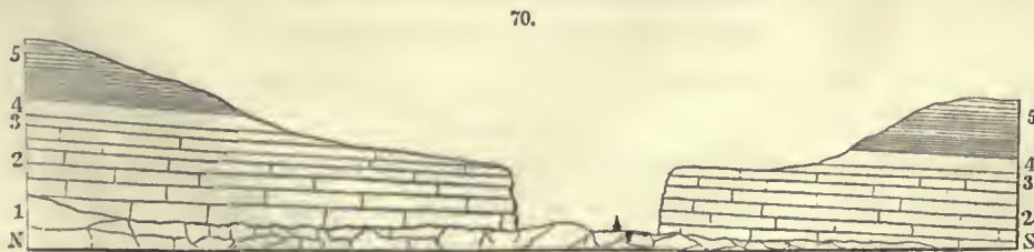
Section north and south, passing through Little-Falls.
