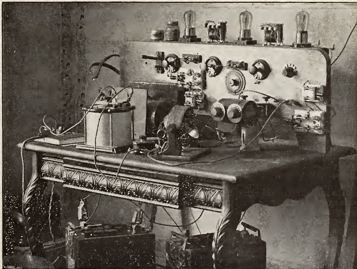
This Radio Regenerative Receiving Set, built by A. C. Philips, Hempstead, N. Y., has proved very effective. The antenna is composed of four strands of solid copper wire spaced two feet, eighty feet long, with a twenty-one foot lead-in. Height 51 feet. A home-made inductance wound on cardboard is used, with movable secondary, and taps on primary. A home-made variometer is used in the circuit as a tickler. The detector and two step amplification is made of standard parts. Double pole double throw switches connect to honey comb coils for long wave lengths. The following stations have been regularly and plainly heard. WJZ—WG1—WBZ—WGY—WWZ—KDKA—WDL—NOF—2XJ—IBKA—WYEB. The layout was arranged after a great deal of experimenting with different makes of standard parts, and left as shown owing to the fact that results were most satisfactory. Six sets of phones connected in series around the receiving room afford convenience and comfort to those who listen in.
