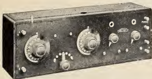
CROSLEY RECEIVER MODEL VI. This set consists of one stage of Tuned Radio Frequency Amplification and Audion Detector. It is normally for use with head phones, but is especially recommended to be used with any type of loud speaker. Additional amplification is unnecessary if head phones and horn are used in receiving local stations. Price without phones, batteries or tubes.....$30.00
