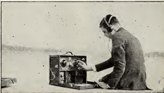
At the sea-shore or away in the mountains it is now possible to be in almost constant communication with the city. This portable radio set has a receiving range of several hundred miles and a transmitting range of four or five miles
