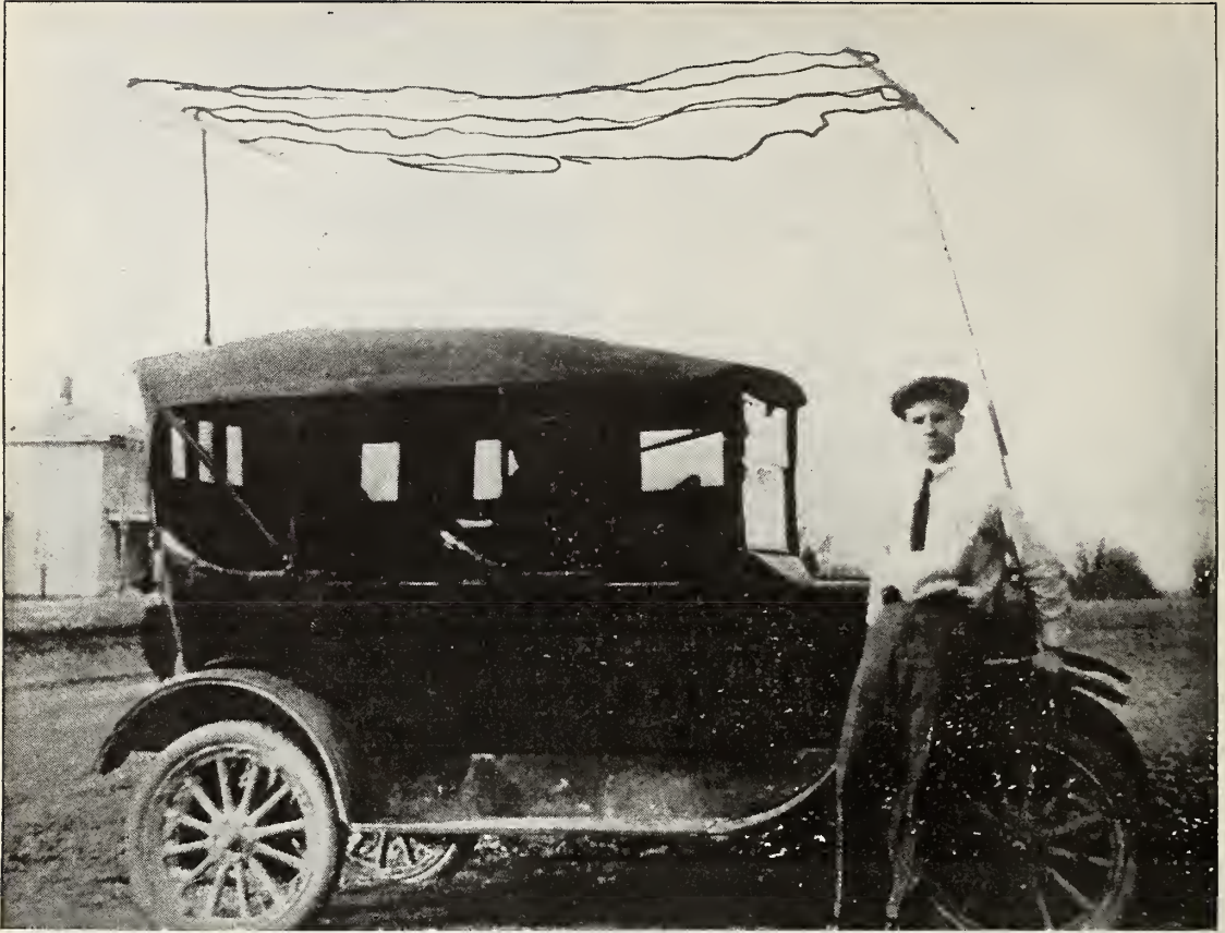
Not pretty, but it works. This radio installation put on his Ford by "Bud," Slocum, a 16-year-old sophomore in Ionia High School, Mich., is not as neat and compact as those to be installed on California's automobile stage lines—but it works
