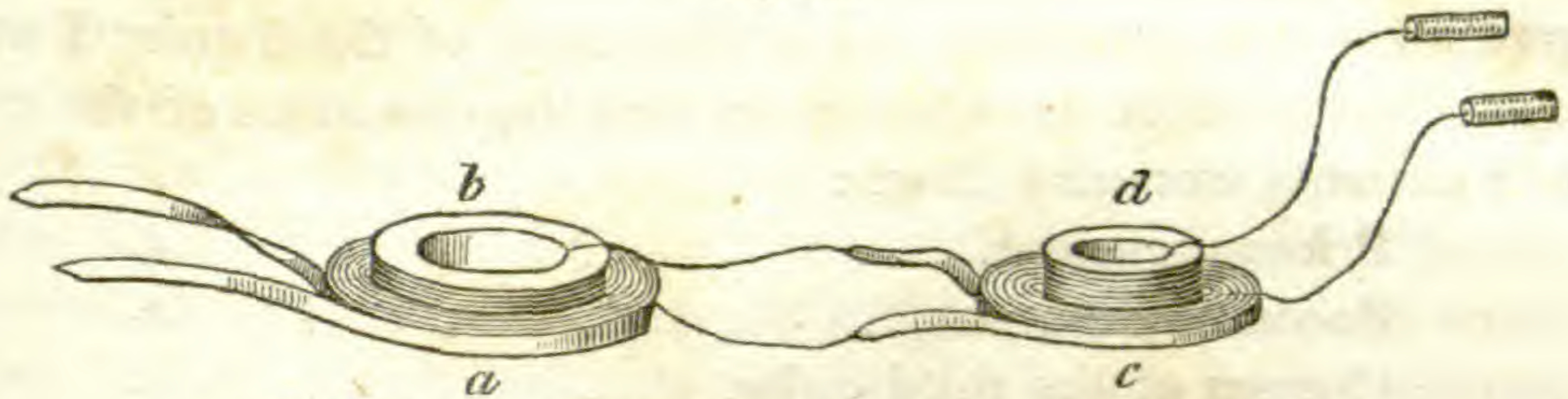
a coil No. 2, b helix No. 1, c coil No. 3, and d helix No. 2.
