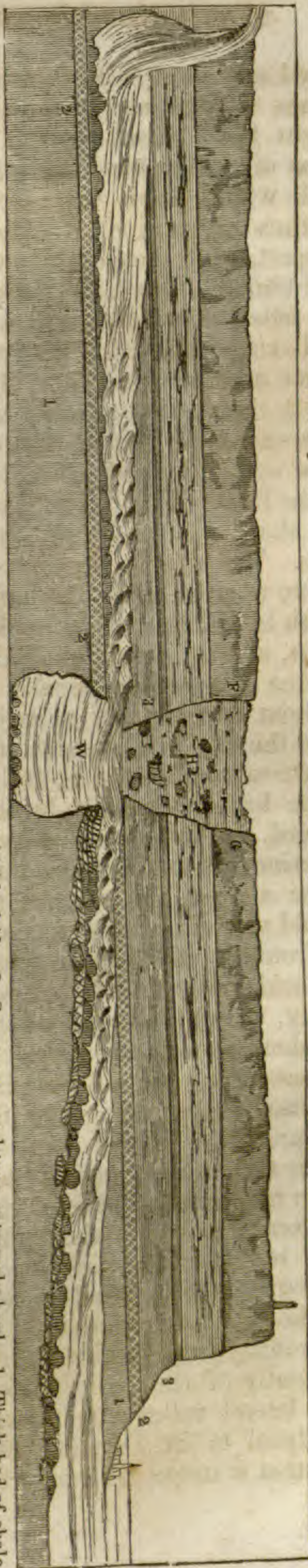
Fig. 2. A Section of the Strata on the Canada side of the Niagara River, from the Falls to Queenston.
