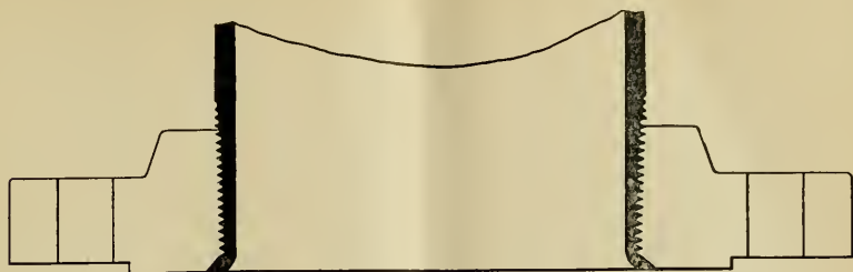
FIG. 10. — ILLUSTRATING A PEENED PIPE.
