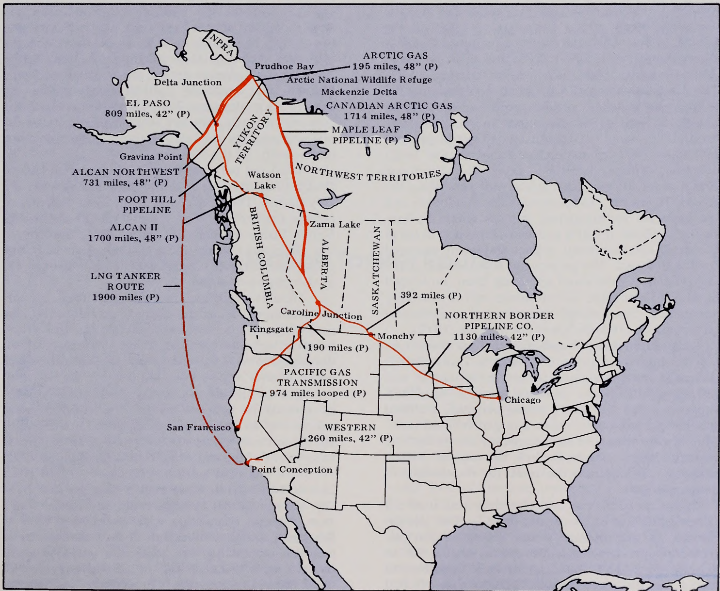
FigureA-21. Proposed (P) Gas Transportation Systems from Alaska to the Conterminous United States.
