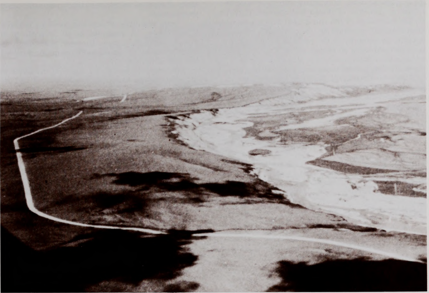
Methods to prevent interference with animal populations were used during construction of the trans-Alaska pipeline. This lateral deviation avoids a peregrine falcon nesting site.
