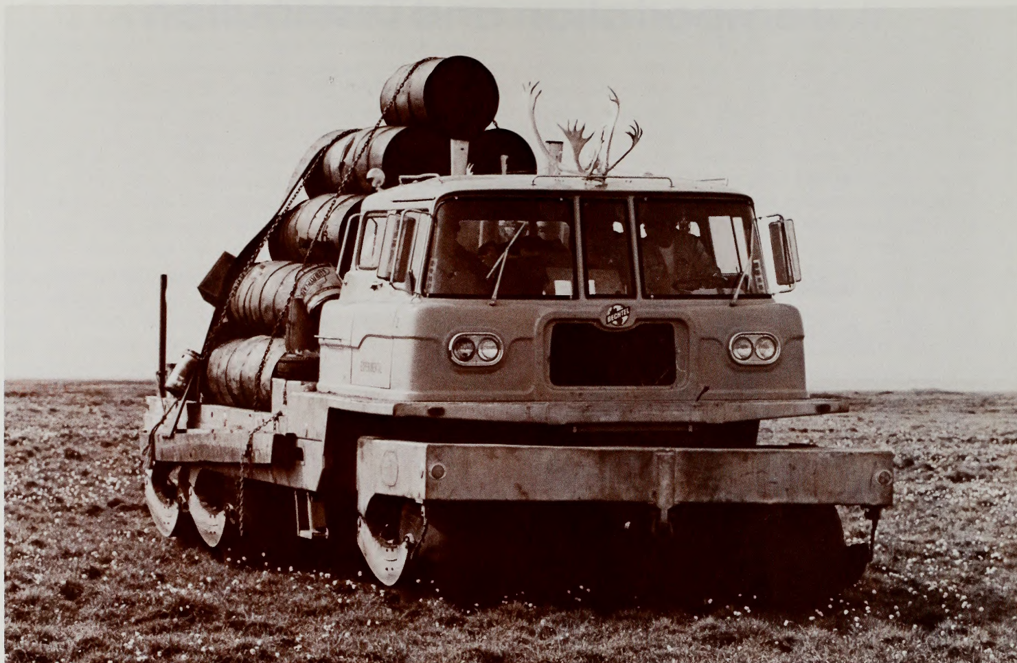
Empty oil barrels at abandoned sites were a scenic eyesore. During recent summers they were removed by clean-up crews using Rolligons. (Atlantic Richfield Company)
